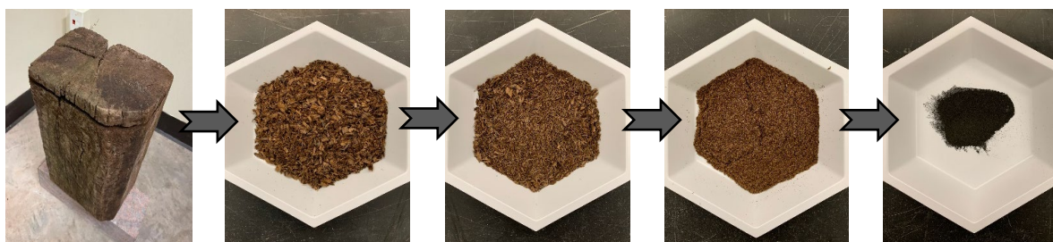
Figure 16. Railroad tie pretreatment. a) Railroad ties biomass, b) sized down RRT, c) dried and grounded, d) sieved biomass to particles size below \mu\text{m} 300, e) produced biochar (sieved for the second time to achieve the desired particle size) for other use proposes.
