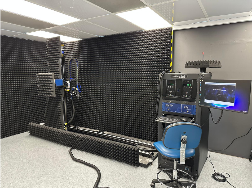
Figure 6.1: Finalized version of the near-field planar scanner (Courtesy: eMWave-tech)
