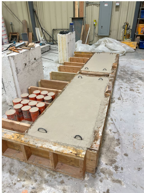
Figure 14: Example Large-Scale Slabs in Formwork
