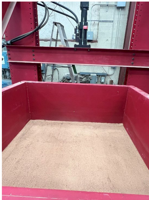
Figure 9: Step 1: Leveled Sand Subgrade in the Soil Containment Box
