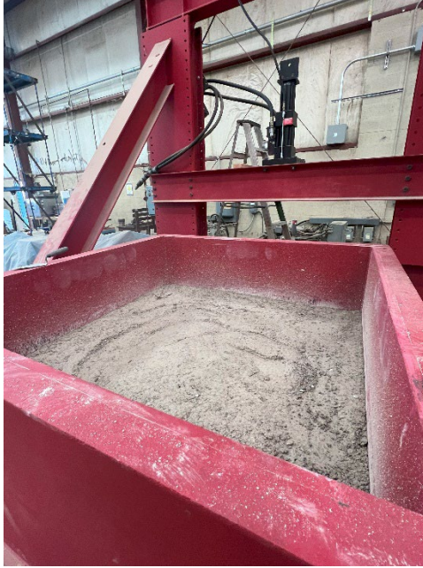
Figure 10: Step 2: Compacted Aggregate Subbase in the Soil Containment Box
