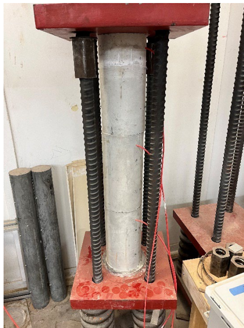
Figure 6: Creep Cylinders Stacked in Loading Frame
