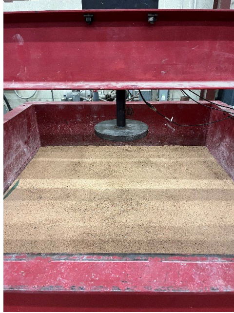
Figure 12: Step 4: Leveled Sand Top Layer Placed in Soil Containment Box
