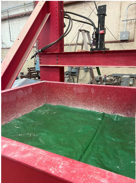
Figure 11: Step 3: Moisture Barrier Placed in the Soil Containment Box
