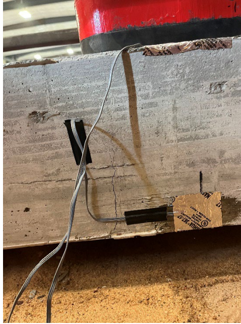
Figure 20: Placement of Foil Strain Gauges on Slab Specimen
