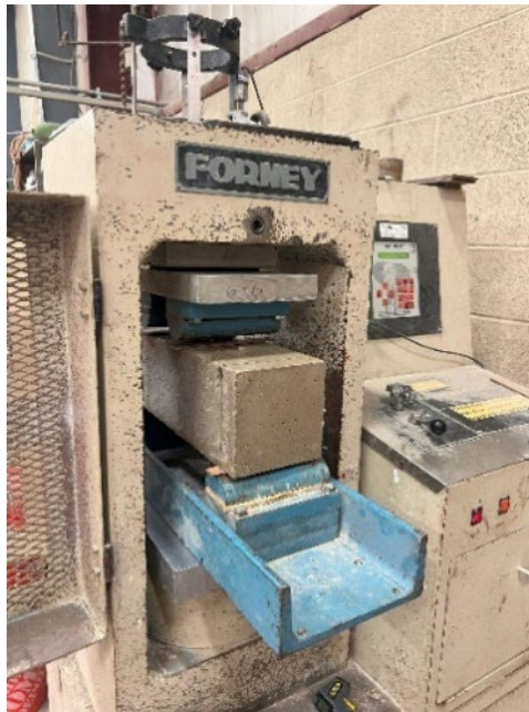
Figure 2: Modulus of Rupture, Third Point Loading
