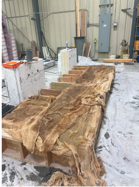
Figure 16: Curing Conditions of OPC Specimens
