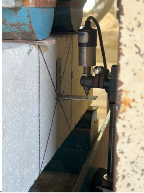
Figure 3: LVDT Placement for 28 Day Modulus of Rupture Testing
