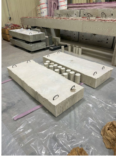
Figure 15: Expansive BCSA Slabs Laid Upon Plastic Lining for Wet-Curing
