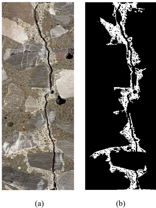
Figure 8: Typical results of the silane products with 90-100% active ingredients and medium silane molecule size. (a) represents a sample after ponding it water. (b) shows the same sample after image processing to show the waterproofing regions around the crack.
