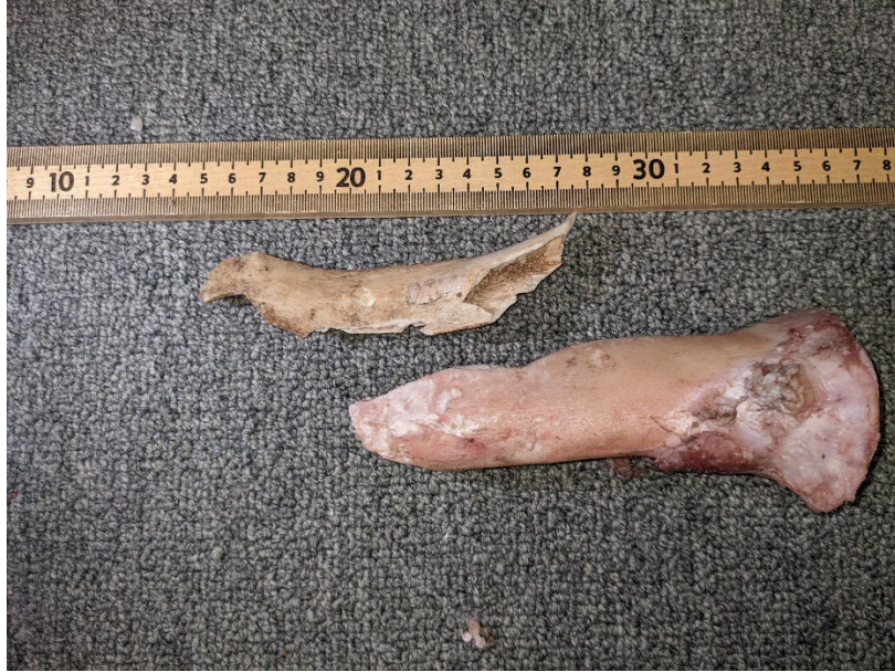
Figure 7-11. Successful experimental radius fracture.
