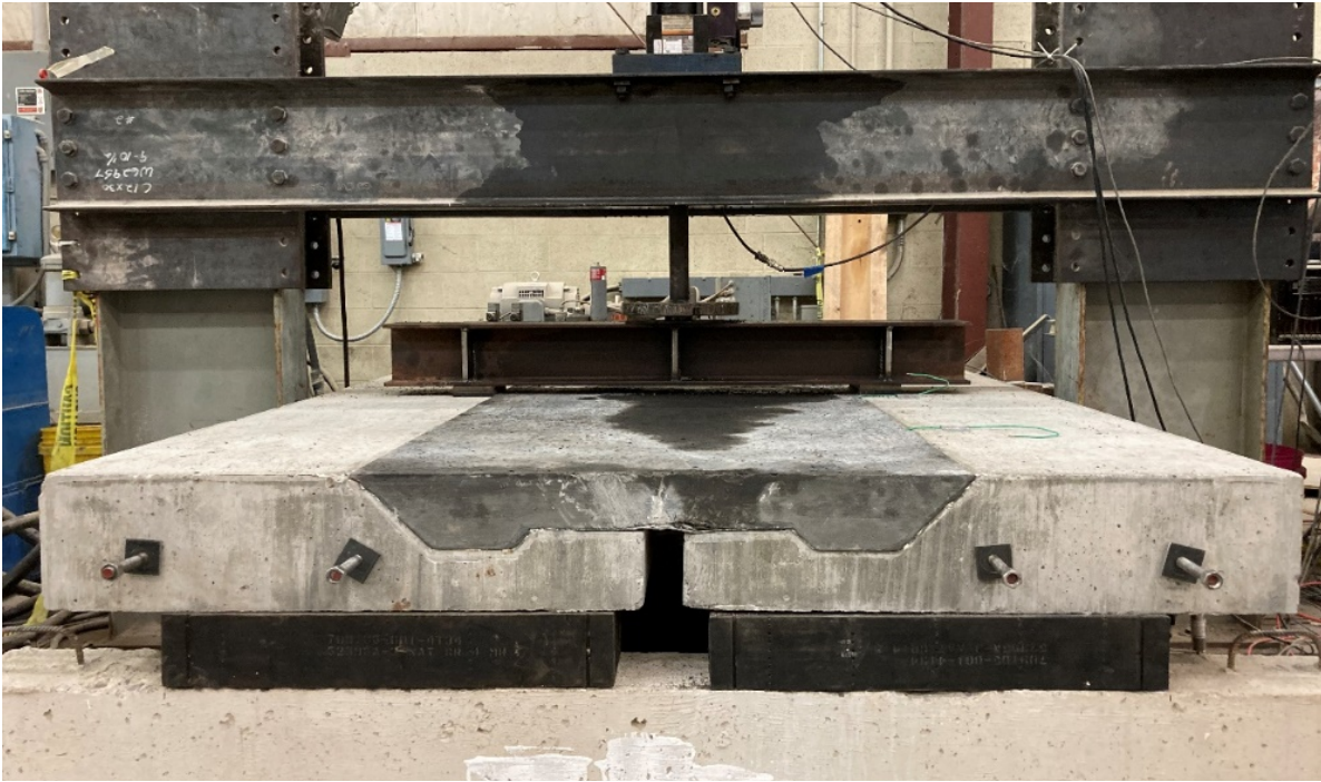
Figure 3-26: Cyclic load testing setup for compression on link slab surface
