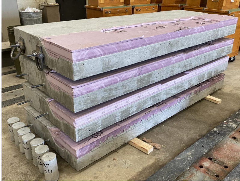
Figure 3-16: Slab sections after demolding, flipping
