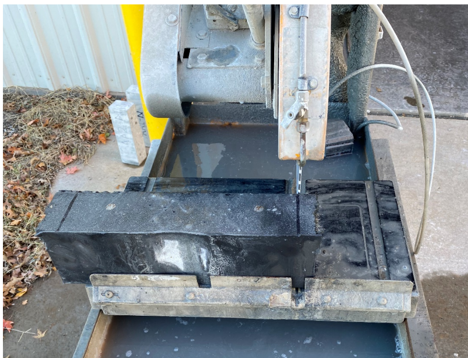
Figure 4-3: Cutting freeze-thaw specimen to length
