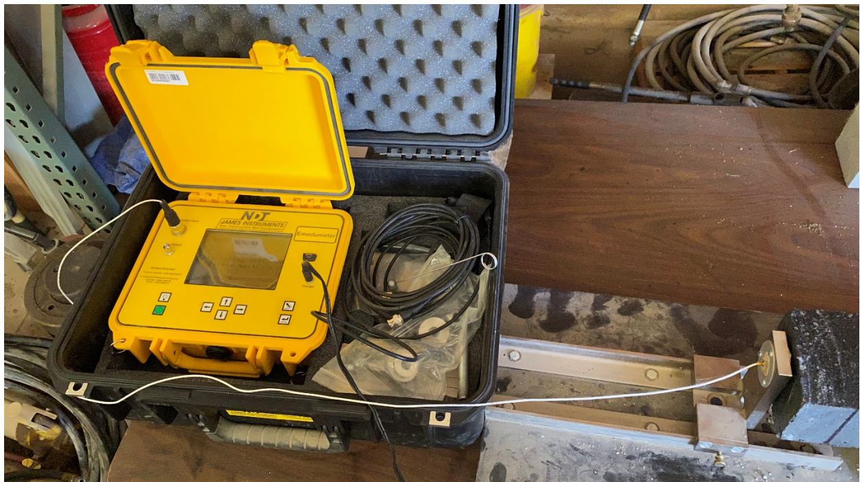
Figure 4-11: Emodimeter with accelerometer connected (white wire)
