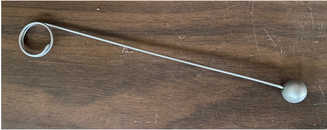
Figure 4-10: Steel impactor used to collect frequency readings
