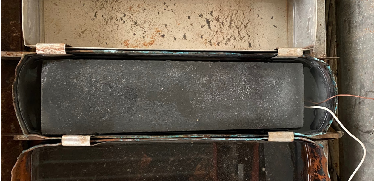
Figure 4-6: Control specimen in freeze-thaw tray
