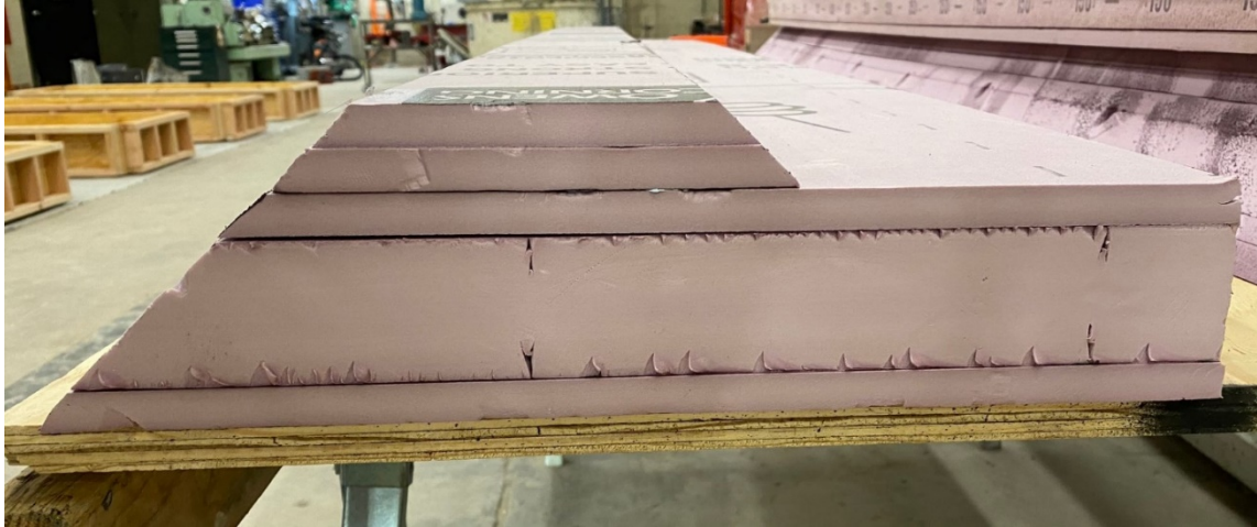
Figure 3-7: Connection cavity foam insert cross-section
