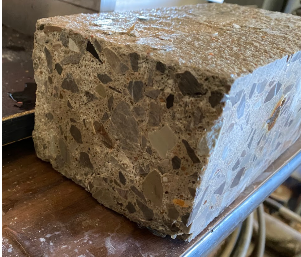
Figure 4-20: Chipped edges, face of specimen AA3-L
