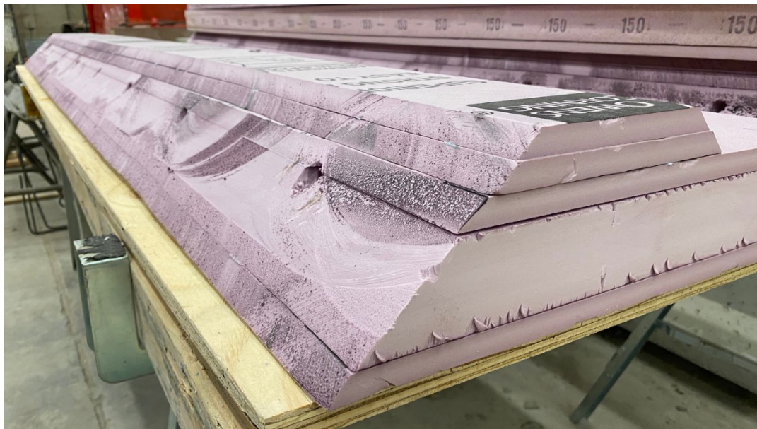
Figure 3-8: Foam insert with drilled holes for rebar
