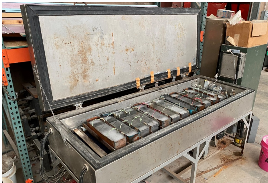
Figure 4-7: Freeze-thaw specimens thawing in cabinet
