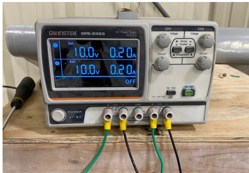
Figure 5-3: DC power supply with test settings
