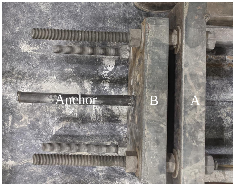
Figure 4-10: Dead end anchor in contact with the prestressing frame
