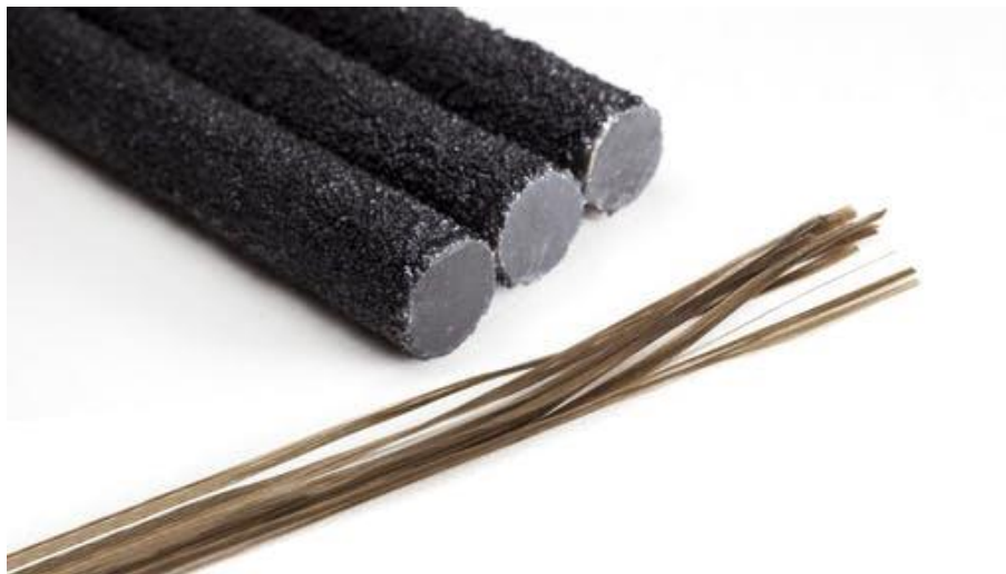
Figure 2-1: Image of a BFRP rebar (Raghavendra Vasudeva Upadhyaya, 2018)
