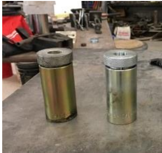
Figure 3-3: Photograph of one set of prestressing chucks used for testing
