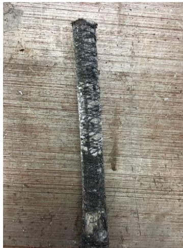
Figure 3-5: BFRP rod after removing the chucks that slipped during testing
