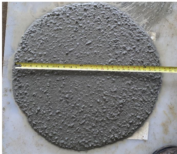
Figure 5-2: Slump flow test for 3 rd concrete mix (slump flow =27 in)
