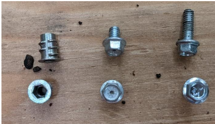
Figure 4-7: From the left to the right: stainless-steel threads, final screw used to read strain from gage, temporary screw
