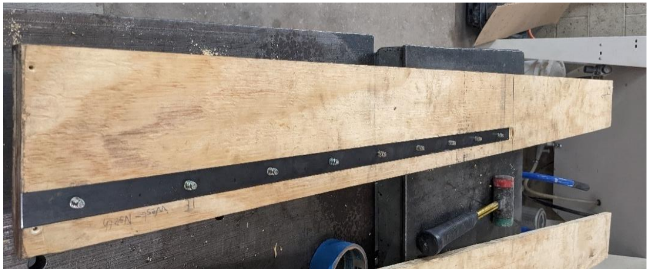
Figure 4-6: Photograph of the steel strip mounted inside one side of the formwork pieces with the internal stainless-steel threads shown
