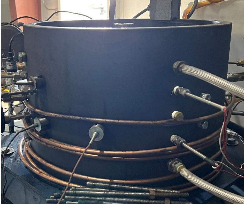
Figure 15: Copper Coils Around the DUT
