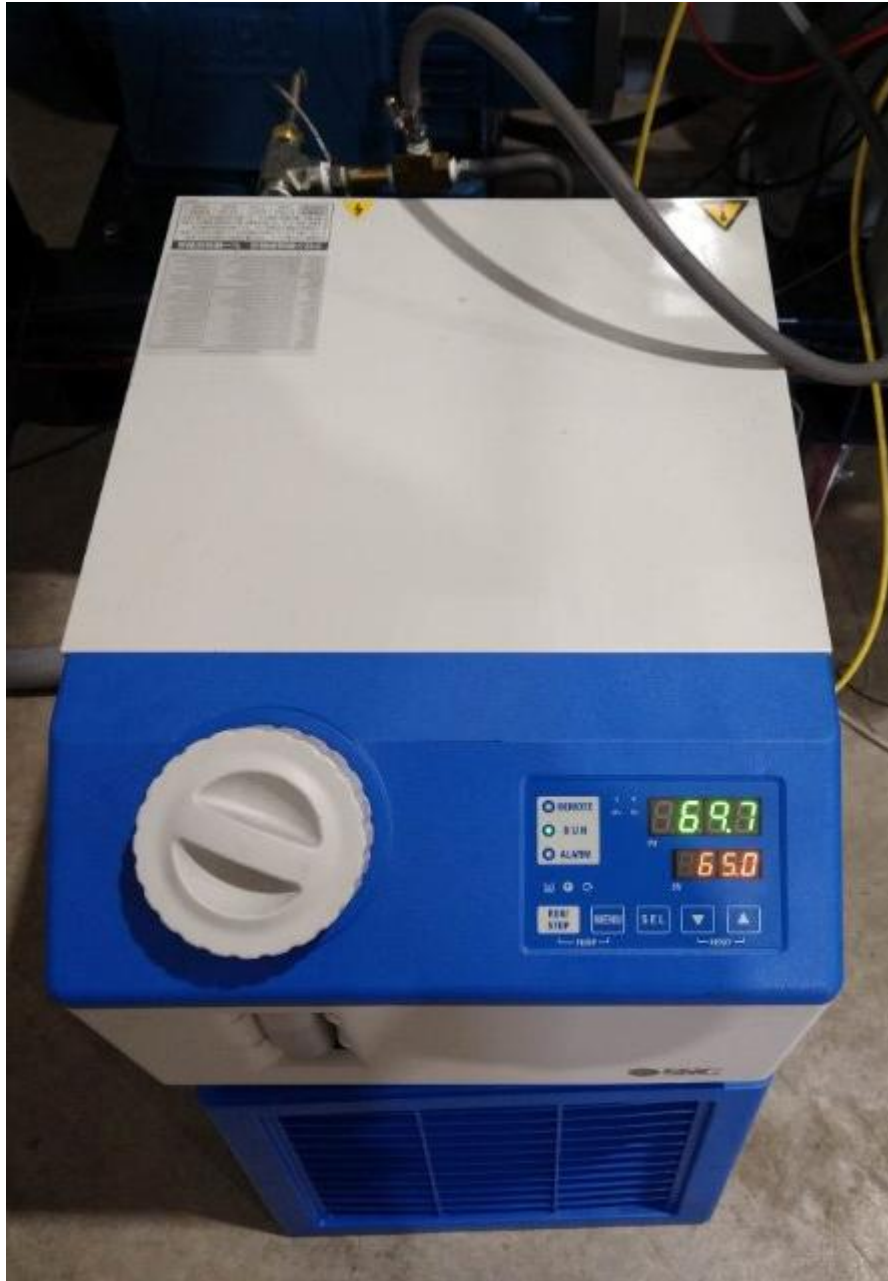
Figure 14: Chiller Added to the Cooling System
