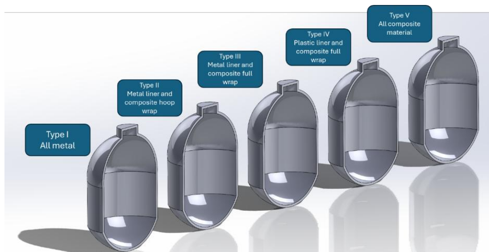
Figure 11: Types of compressed hydrogen gas storage tanks [17].
