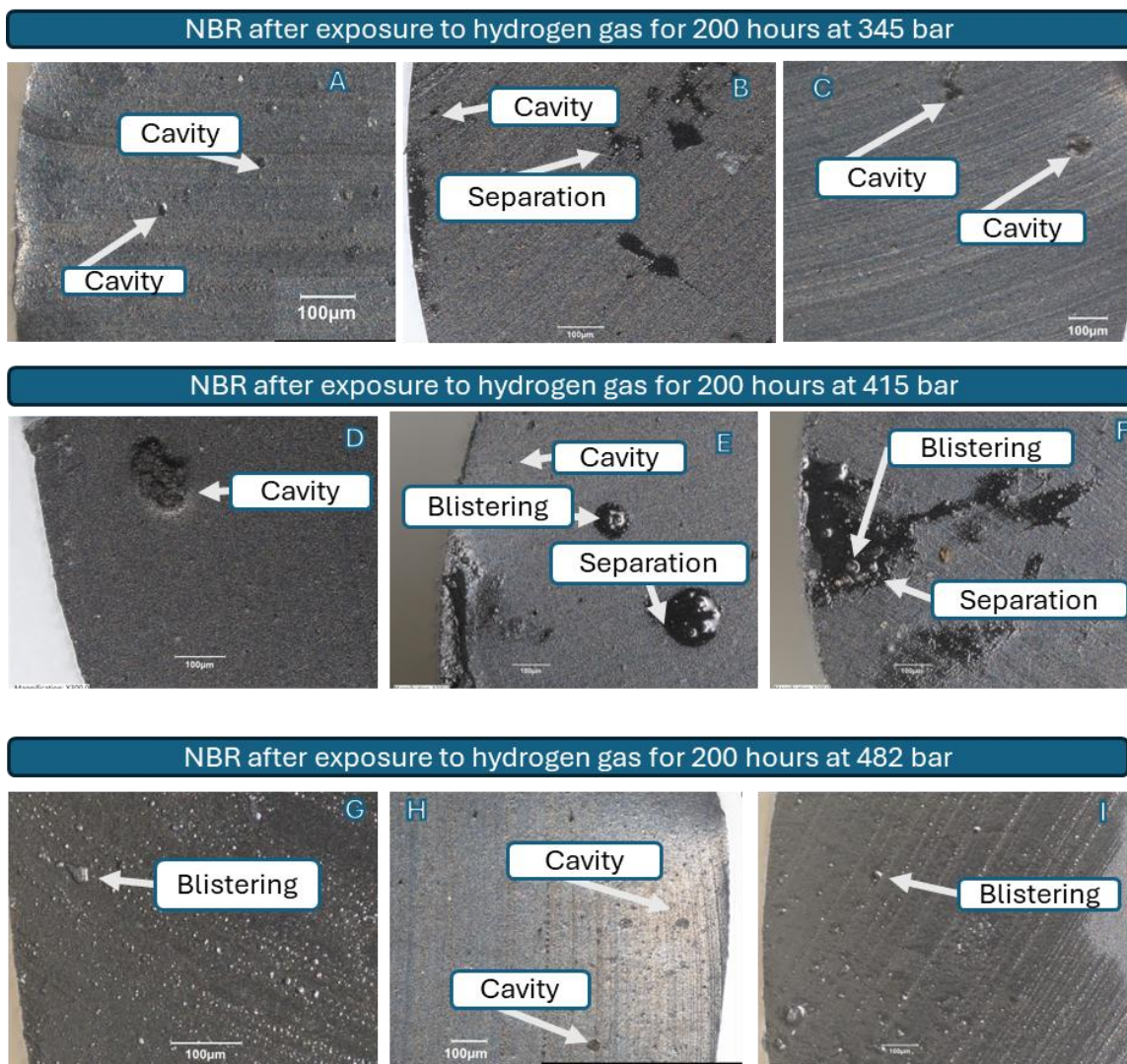
Figure 63: Microscopic images obtained from NBR O-ring samples exposed to hydrogen gas at 345 bar 415 bar and 482 bar respectively highlighting the main defects observed.
