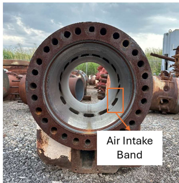
Figure 1: Combustion Chamber Design with Air intake Cutouts
