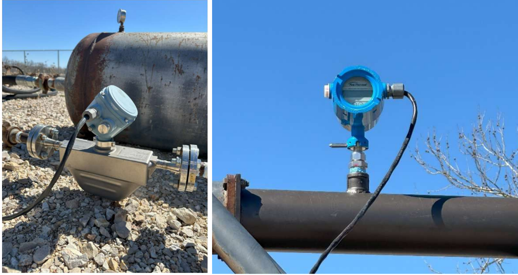
Figure 9: Flow meters used in experimentation, (a) Emerson flow meter for natural gas stream, (b) Fox Thermal flow meter for air and/or hydrogen data collection.
