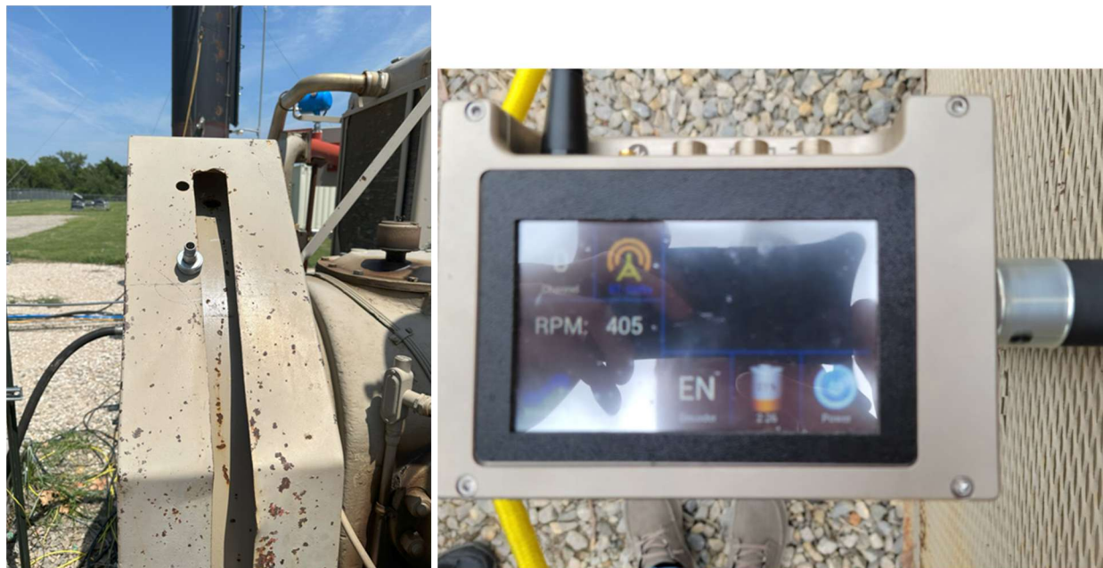
Figure 12: (a, left) Permanent Magnetic RPM Encoder, (b, right) Windrock Magnetic Encoder
