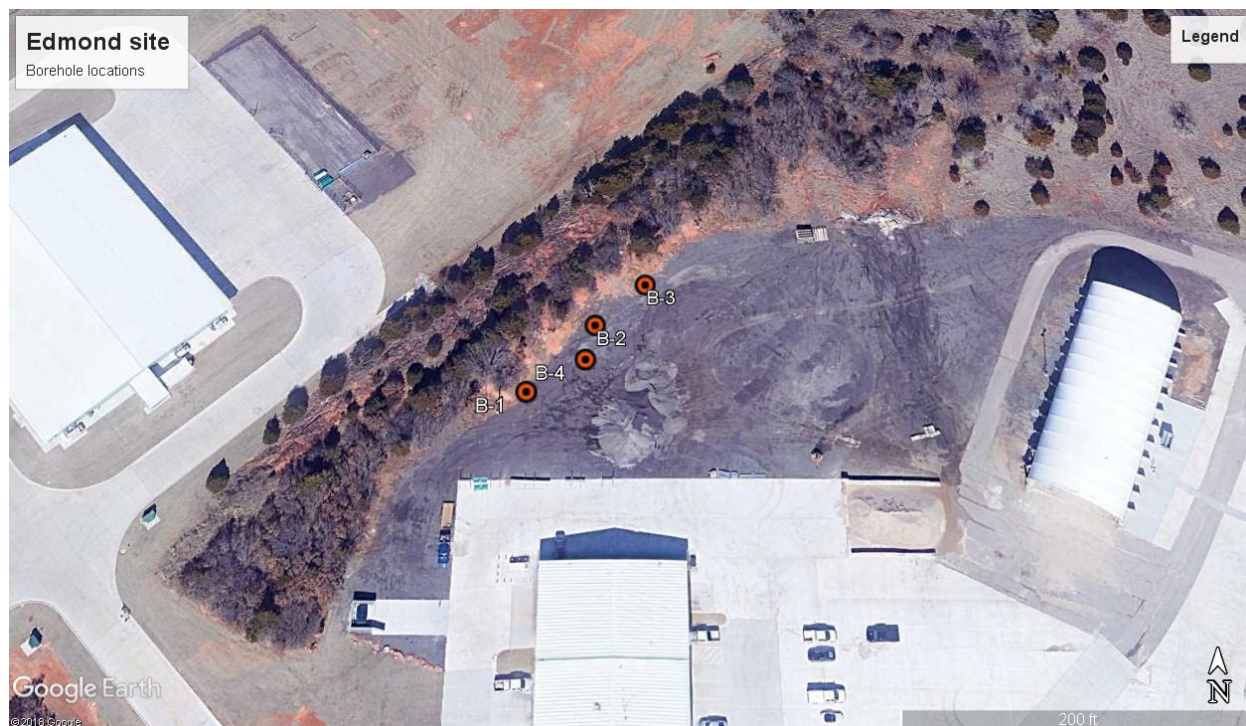
Figure 3.1 – Aerial photo of Edmond test site showing boring locations.
