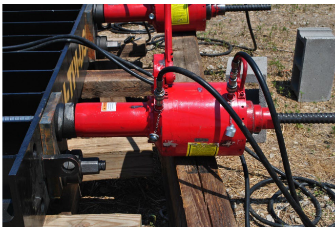
Figure 7.13 – Hydraulic jack on threaded bar applying load to beam through a bearing plate.
