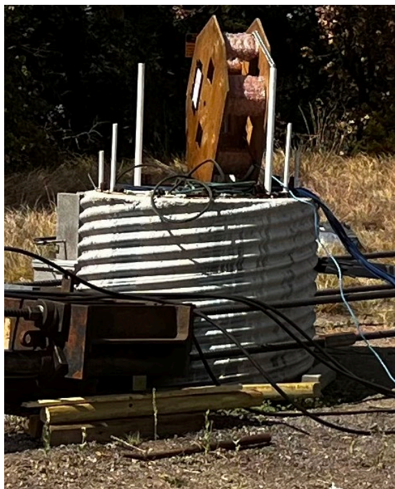
Figure 7.9 – ShapeArray resting atop Edmond T3 during testing.
