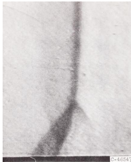
Figure 3. Mark's experimental visualization of reflected shockwave bifurcation in a shock tube [15].
