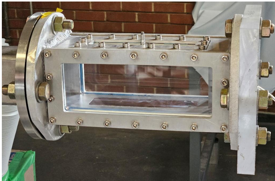
Figure 8. Completed test section installed in the HSAL shock tube facility. The viewpoint is from the left-hand side of the test section.
