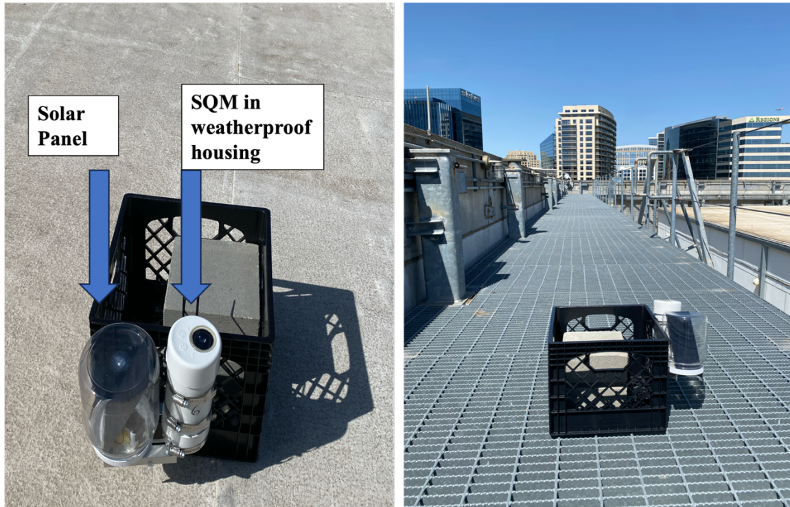
Figure 1.3. Sky Quality Meter LU-DL mounted to weighted milk crate and deployed on host location rooftop.
