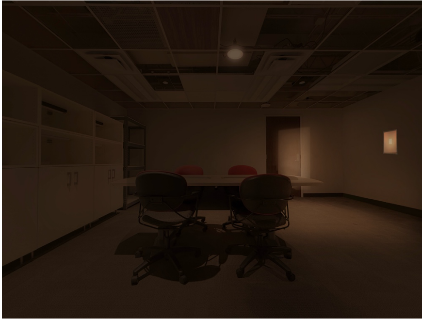
(a) 2200 K, spotlight tilted 30° toward the west wall, 300 lm
