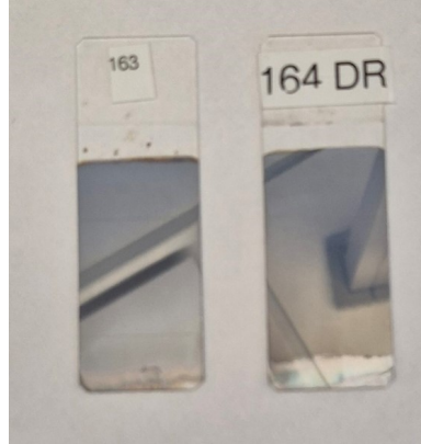
Fig. 2.12: Single Layer (left) and Double Layer (right) PbSe thin Film deposition using CBD method
