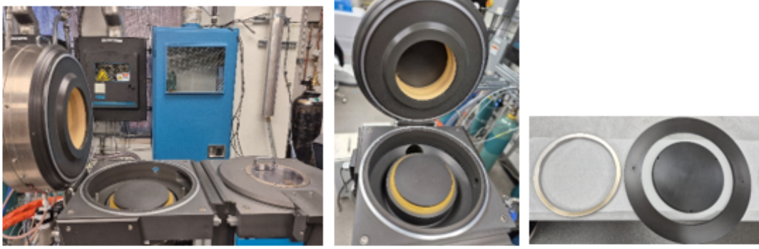
Fig. 4.8: Cleaning of Reactive Ion Etching reactor chamber
