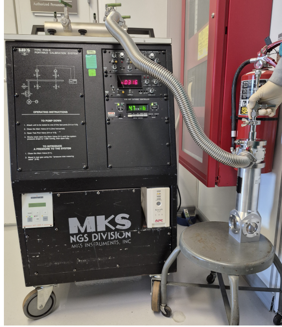
Fig. 4.13: Turbomolecular pump used to achieve vacuum in cryogenic at lower pressures
