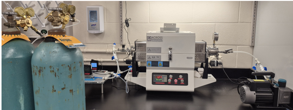
Fig. 3.3: Thermal annealing treatment setup
