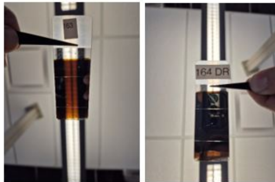
Fig. 2.13: Single Layer (left) and Double Layer (right) PbSe thin Film deposition under the light
