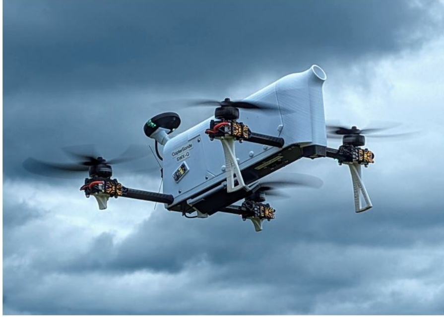
Figure 2.2: The CopterSonde-SWX (CSWX), developed in 2024, represents the next evolution of weather-sensing UAS technology, extending the capabilities of the earlier CopterSonde-3D platform. Developed for deployment in severe weather environments, the CSWX incorporates an advanced aerodynamic design tailored to enhance flight stability and improve measurement accuracy under high-wind atmospheric conditions.
