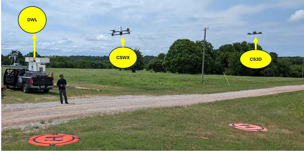
Figure 4.1: Field deployment setup showing the CS3D and CSWX UAS platforms operating in coordination with the DWL system at the KAEFS site. Both CopterSonde platforms ascended to altitudes of up to 1000 m and were flown simultaneously, maintaining an approximate lateral separation of 10 m from each other and 20 m from the DWL unit.
