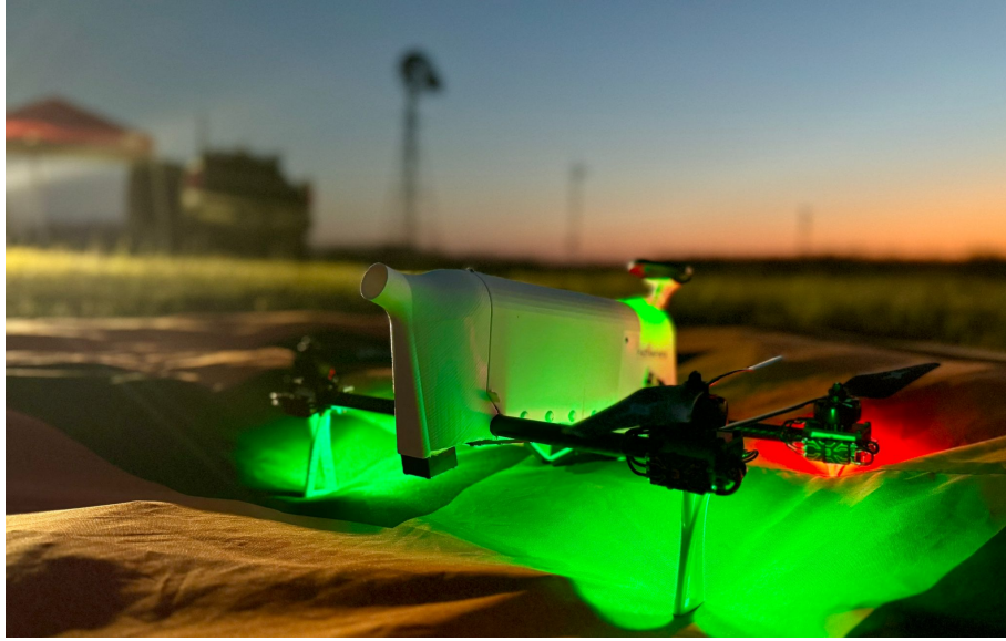
Figure 2.3: Side view of the CSWX on the launchpad after a night flight, illustrating the platform’s streamlined airframe designed to enhance aerodynamic efficiency and operational stability in high-wind environments.
