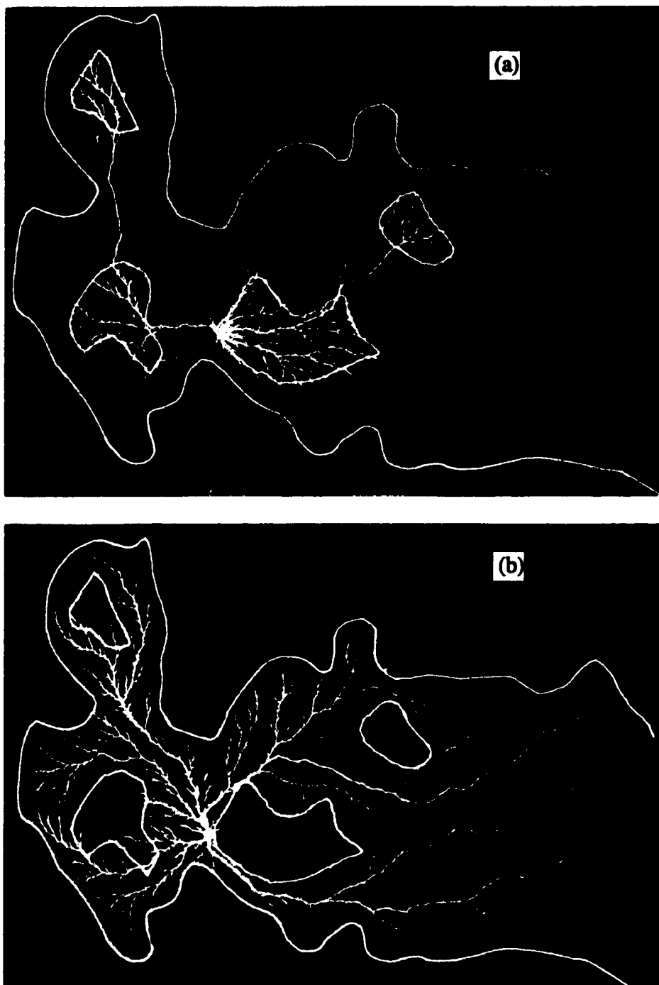
Figure 4.5: Discharges through plastic with two charge densities. (a) Isolated regions of higher charge density ( -1.2 \text{ C m}^{-3} ) are surrounded by lower charge density ( -0.6 \text{ C m}^{-3} ). (b) Isolated regions of lower charge density ( -0.6 \text{ C m}^{-3} ) are surrounded by higher charge density ( -1.2 \text{ C m}^{-3} ). Reproduced from Williams et al. 1985, Figure 6.
