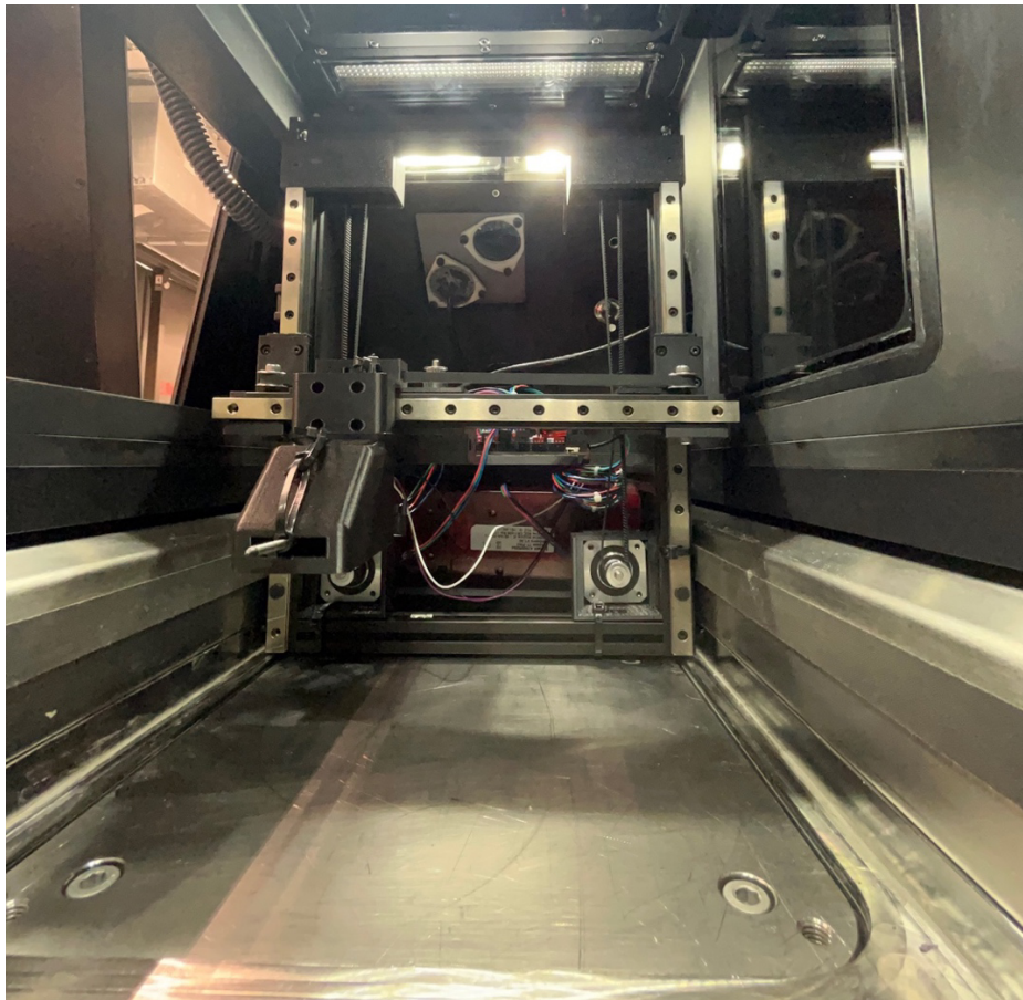
Figure 16. Final airflow measurement device fully assembled in the build chamber (frontal view)
