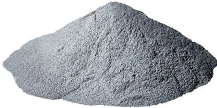
Figure 3. Ti-6Al-4V LPBF printing powder [5]
