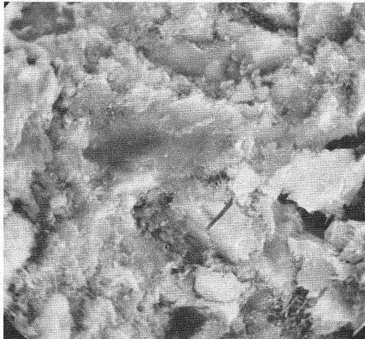
Figure A-15. Fracture Surface of Revibrated Cement Paste After 7 Days of Hydration (X-3).
