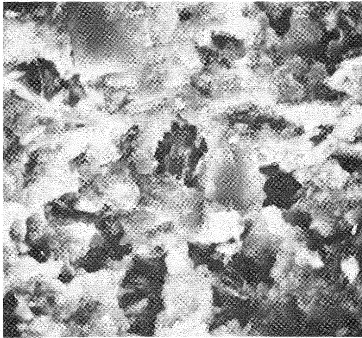
Figure A-13. General View of Fracture Surface of Revibrated Specimen (X-2).
