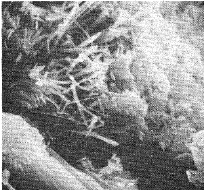
Figure A-14. Calcium Silicate Hydrate in Revibrated Specimen (X-2).
