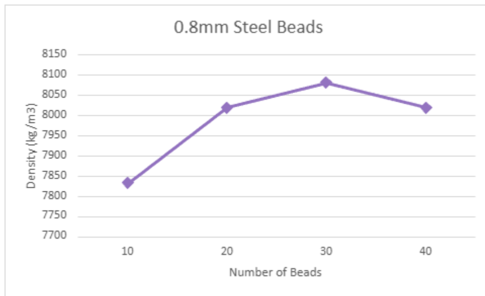
Figure 2.6: 0.8mm Density vs Number of Beads
