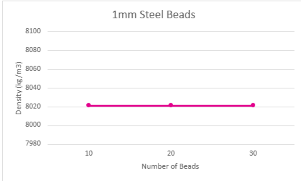
Figure 2.7: 1mm Density vs Number of Beads
