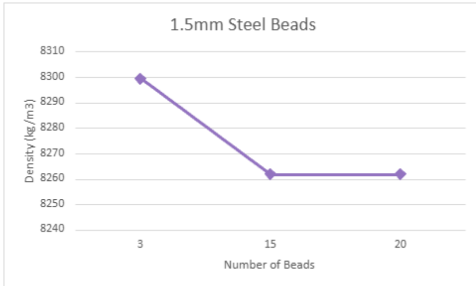
Figure 2.8: 1.5mm Density vs Number of Beads
