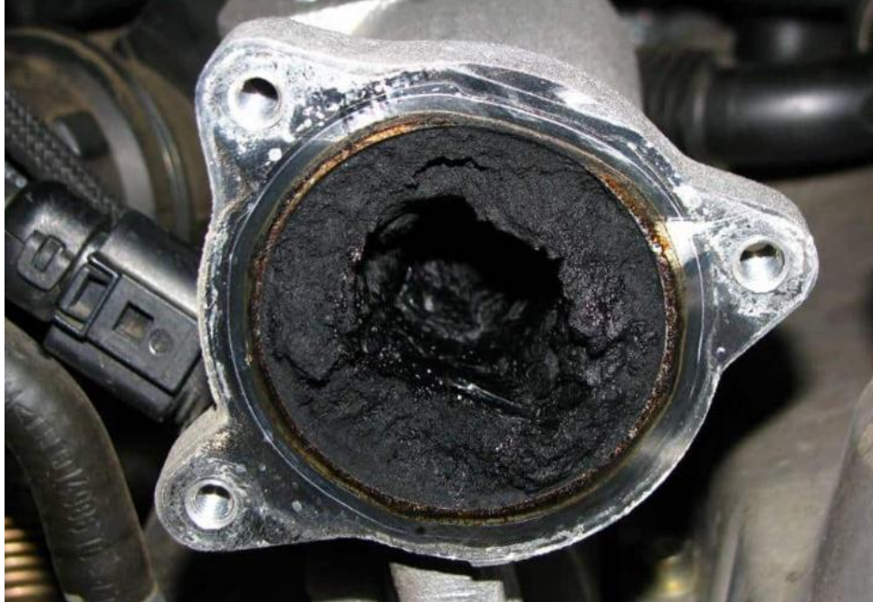
Figure 1: Soot Build-Up in the Exhaust Manifold of a Diesel Engine [3]
