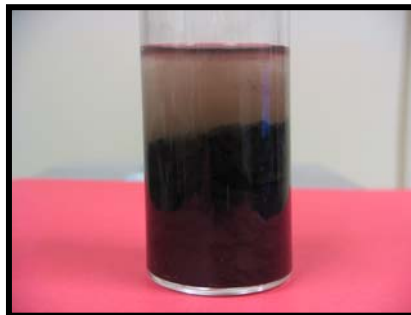
Figure 5.6.1: Crushed shale sample (X749.2 ft) in the form of cuttings immersed in water.
