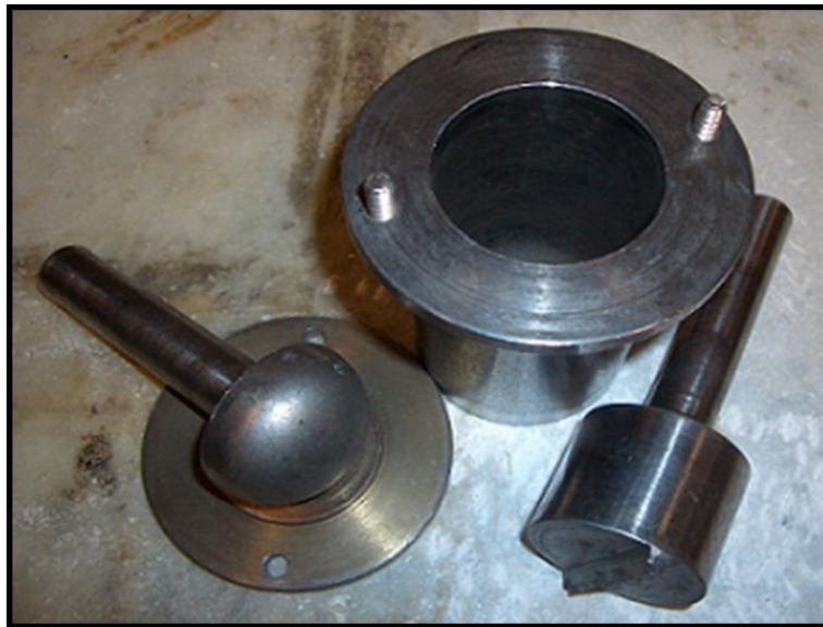
Figure H.1: Covered crucible to crush shale samples. Allows crushing the sample without loss of material.
