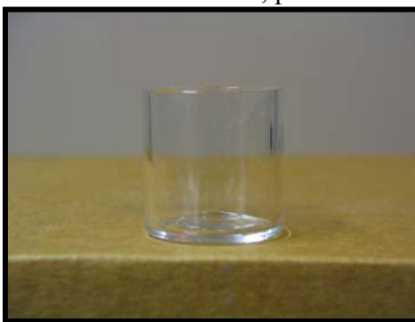
Figure 4.8.1: Empty Glass Vial (Internal Diameter = 1.0” and Height = 1.2”)
