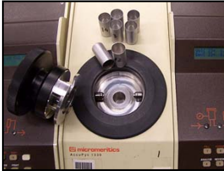
Figure H.2: Low pressure pycnometer (LPP) and aluminum measuring vial.
