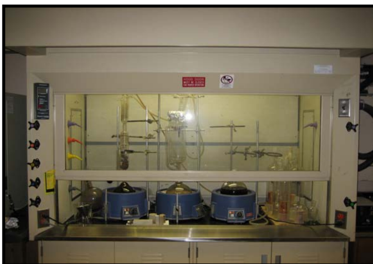
Figure 3.2.1: Soxhlet extractor used to cleaning core samples. Boiling flask filled with 20% methanol and 80% toluene by volume mixture.
