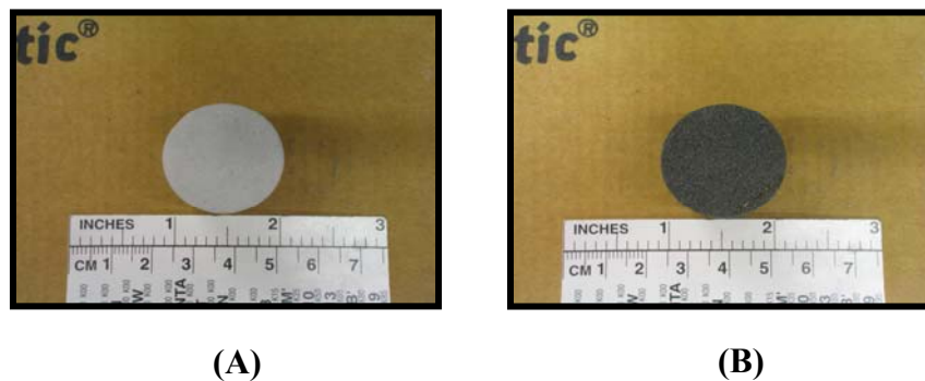
Figure 4.8.6: (A) Filtros, porosity and permeability are 35% and 5D. (B) Kellundite, porosity and permeability are in the same ranges.
