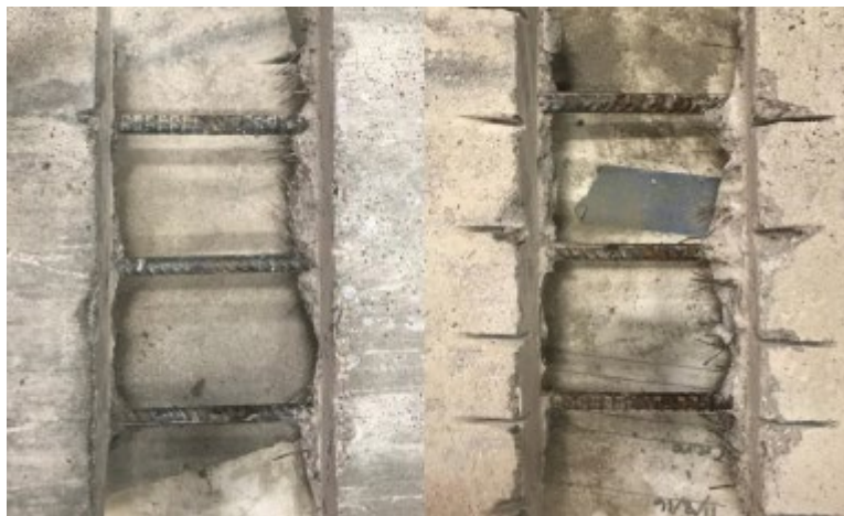
Figure 295. Corrosion state of rebar reinforcing at joint of Phoscrete small-scale corrosion specimens with 4% NaCl (left) and 8% NaCl (right)
