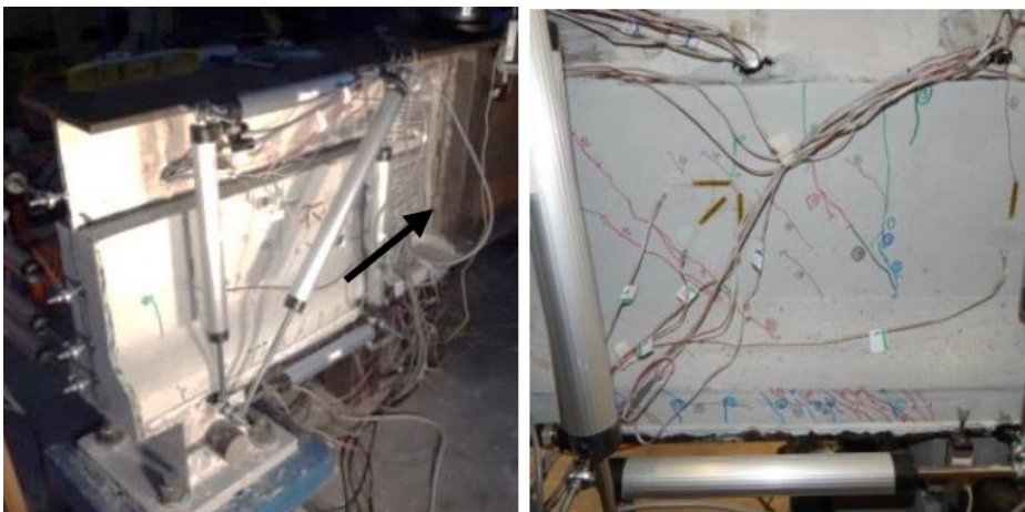
Figure 15. Repaired girder failure (Zmetra 2015)
