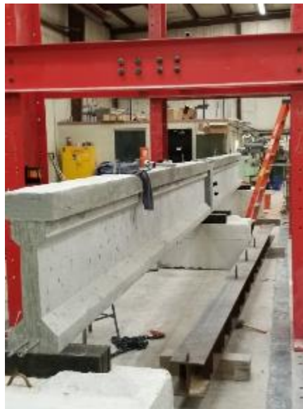
Figure 195. Continuity joint specimen in place for testing
