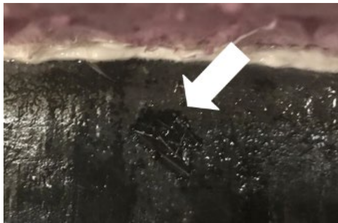
Figure 287. Visual pocketing on Ductal® specimen - 50 cycles
