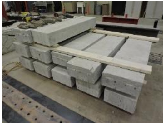
Figure 297. Large-scale corrosion joint specimens before chipping
