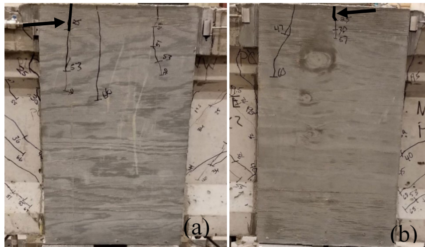
Figure 240. Initial continuity joint flexural cracking on the east face (a) and west face (b) at 25 kips of load. Arrows point to the dark lines that indicate the initial flexural cracks.
