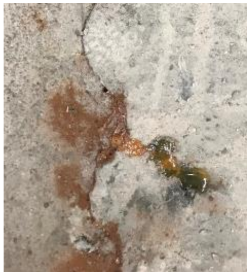
Figure 309. Green liquid in joint of Ductal® large-scale corrosion specimen during week 10 of testing
