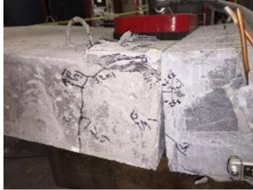
Figure 114. Ductal® slab joint 3 after completion of testing showing concrete crushing and separation at joint indicative of rebar failure
