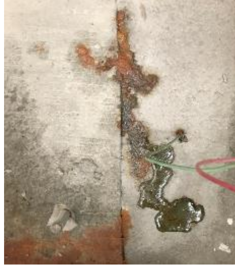
Figure 308. Green liquid in joint of Phoscrete large-scale corrosion specimen during week 10 of testing
