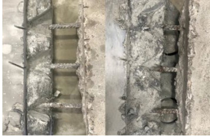
Figure 293. Corrosion state of rebar reinforcing at joint of J3 small-scale corrosion specimens with 4% NaCl (left) and 8% NaCl (right)
