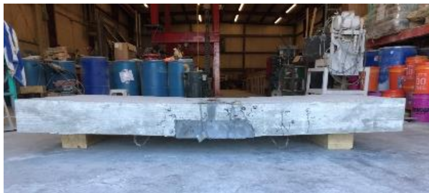
Figure 129. J3 Slab joint 1 curvature after failure
