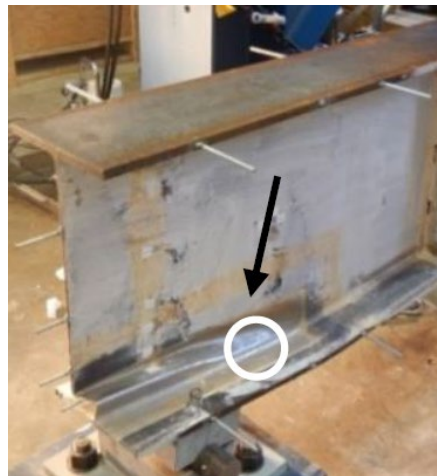
Figure 14. Damaged girder failure (Zmetra 2015)
