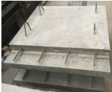
Figure 97. Completed half-depth slab specimens showing protruding rebar
