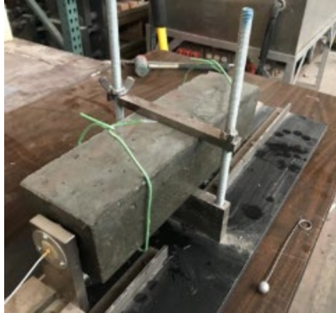
Figure 272. Freeze-thaw specimen arranged for dynamic modulus testing
