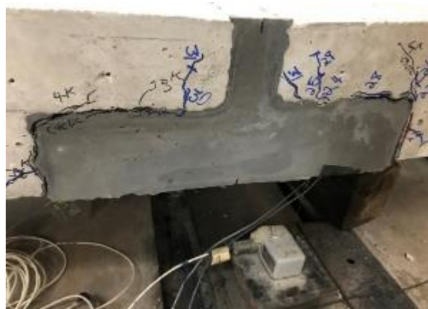
Figure 136. Cracks formed at the conventional concrete to UHPC interface and propagating upward on the south side of J3 slab joint 2
