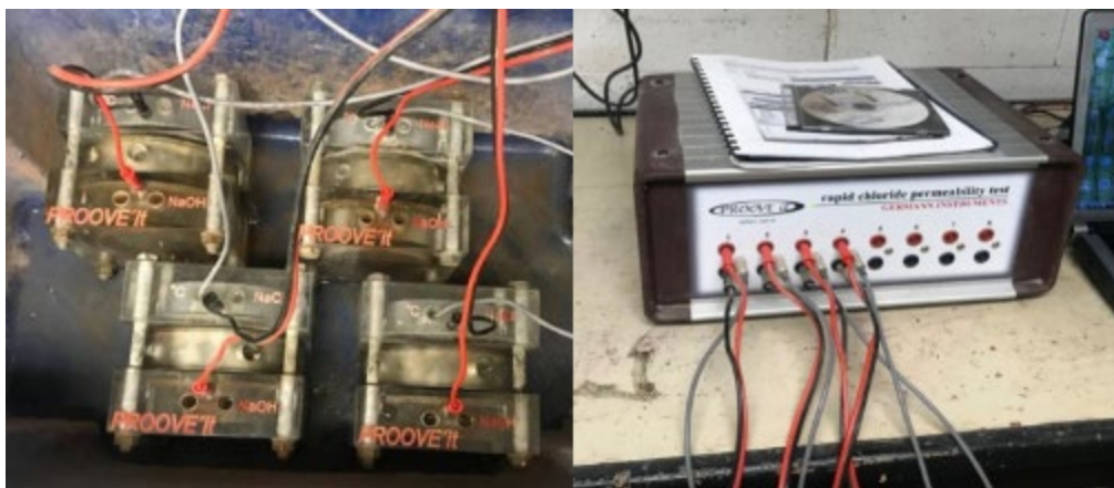
Figure 271. Typical RCIP testing showing test cells (left) and PROOVE'it apparatus (right)
