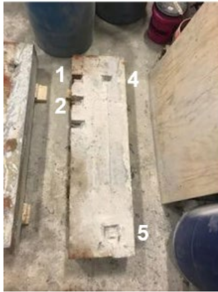
Figure 312. Chipping sequence of large-scale corrosion specimens
