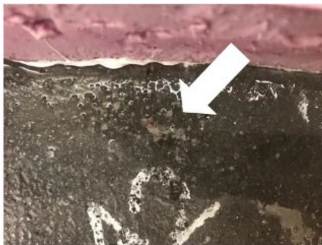
Figure 283. Visual pocketing on AA specimen - 25 cycles
