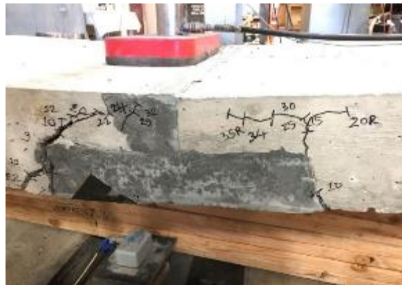
Figure 152. Cracks on the north side of Ductal® slab joint 2 after part 2 testing
