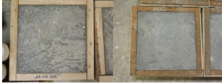
Figure 61. Pull-off test specimens for Ductal® (left) and J3 (right)
