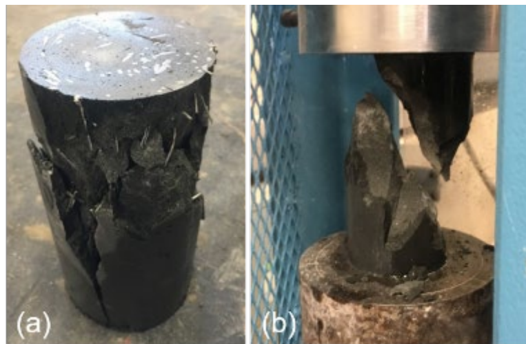
Figure 40. Fiber reinforced (a) and unreinforced specimens after compression testing
