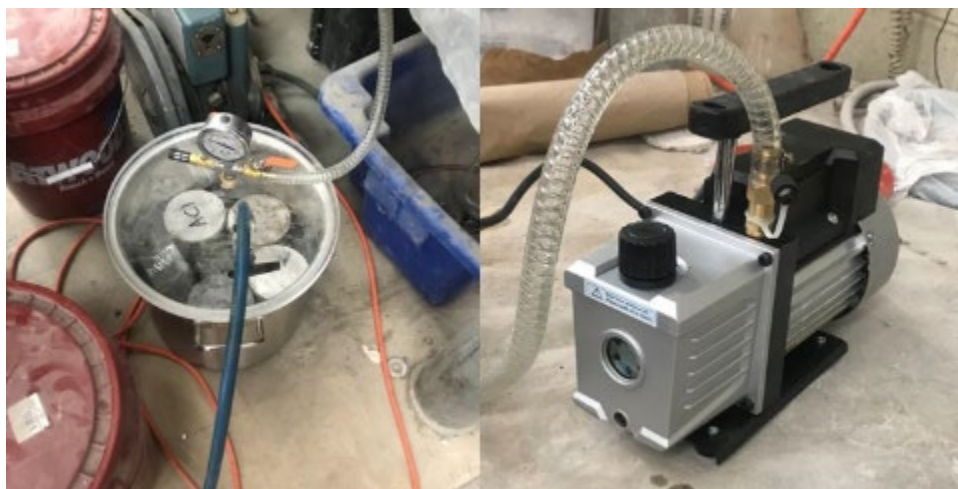
Figure 270. Vacuum desiccator (left) and pump (right) used for RCIP specimen preparation
