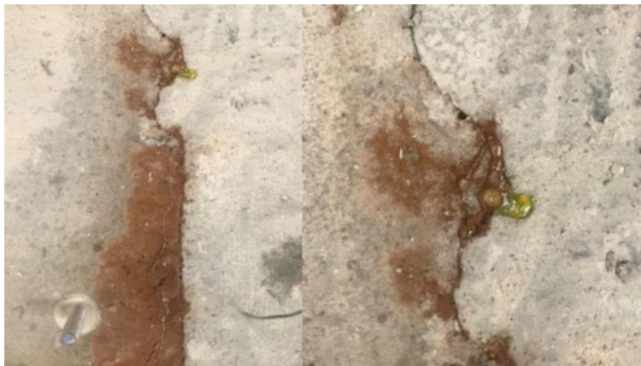
Figure 307. Green liquid in joint of Ductal ® large-scale corrosion specimen during week 8 of testing
