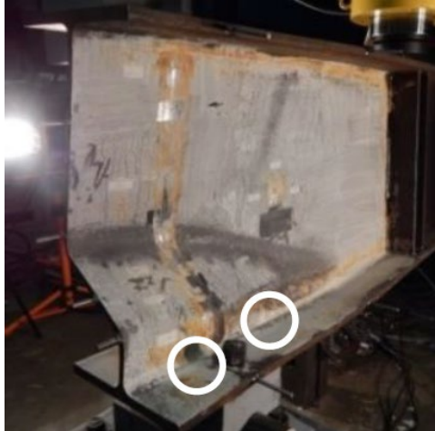
Figure 13. Undamaged girder failure (Zmetra 2015)
