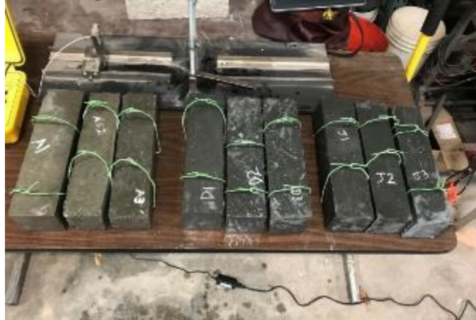
Figure 276. Condition of all freeze-thaw specimens - Cycle 0
