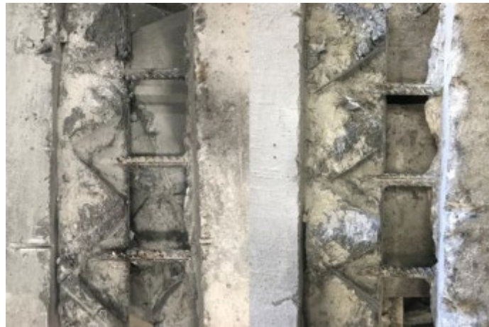
Figure 294. Corrosion state of rebar reinforcing at joint of Ductal® small-scale corrosion specimens with 4% NaCl (left) and 8% NaCl (right)
