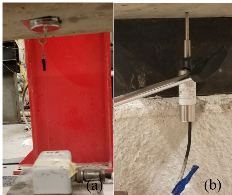
Figure 191. Wire potentiometer (pot) attached to bottom of girder at midspan (a) and linear voltage differential transformer (LVDTs) placed under girder near the support (b).
