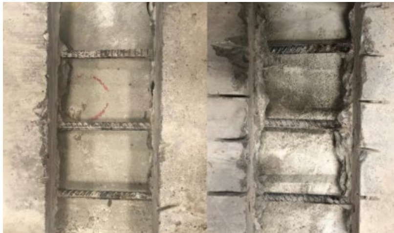
Figure 292. Corrosion state of rebar reinforcing at joint of ODOT Class AA small-scale corrosion specimens with 4% NaCl (left) and 8% NaCl (right)
