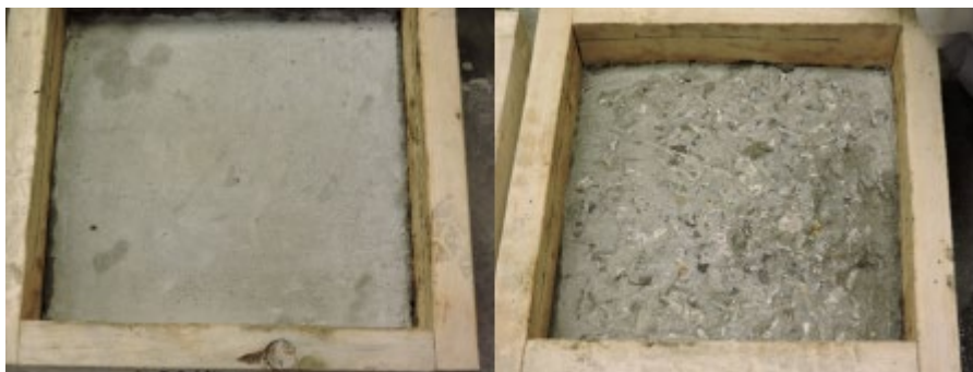
Figure 60. Sandblasted (left) and chipped (right) surface preparations
