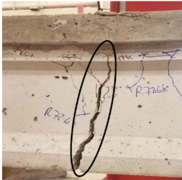
Figure 201. Flexural crack where the prestressing strands ruptured under the load point on the NC1-S girder, indicated by a dark oval
