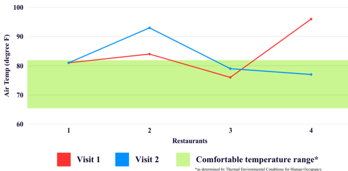
Figure 5. Air Temperature Readings Across Restaurants
