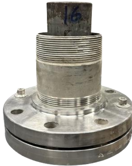
Figure 24: Schematic of the Mold assembly for the shear bond testing.
