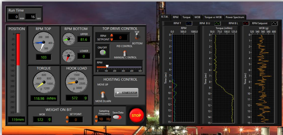
Figure 3-19 A snippet of the HMI (Human machine interface) for the experimental setup
