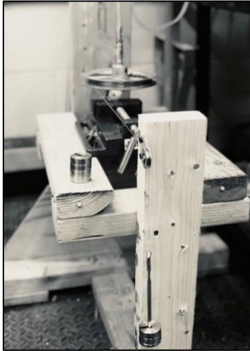
Figure 3-16 Experimental calibration of torque sensor
