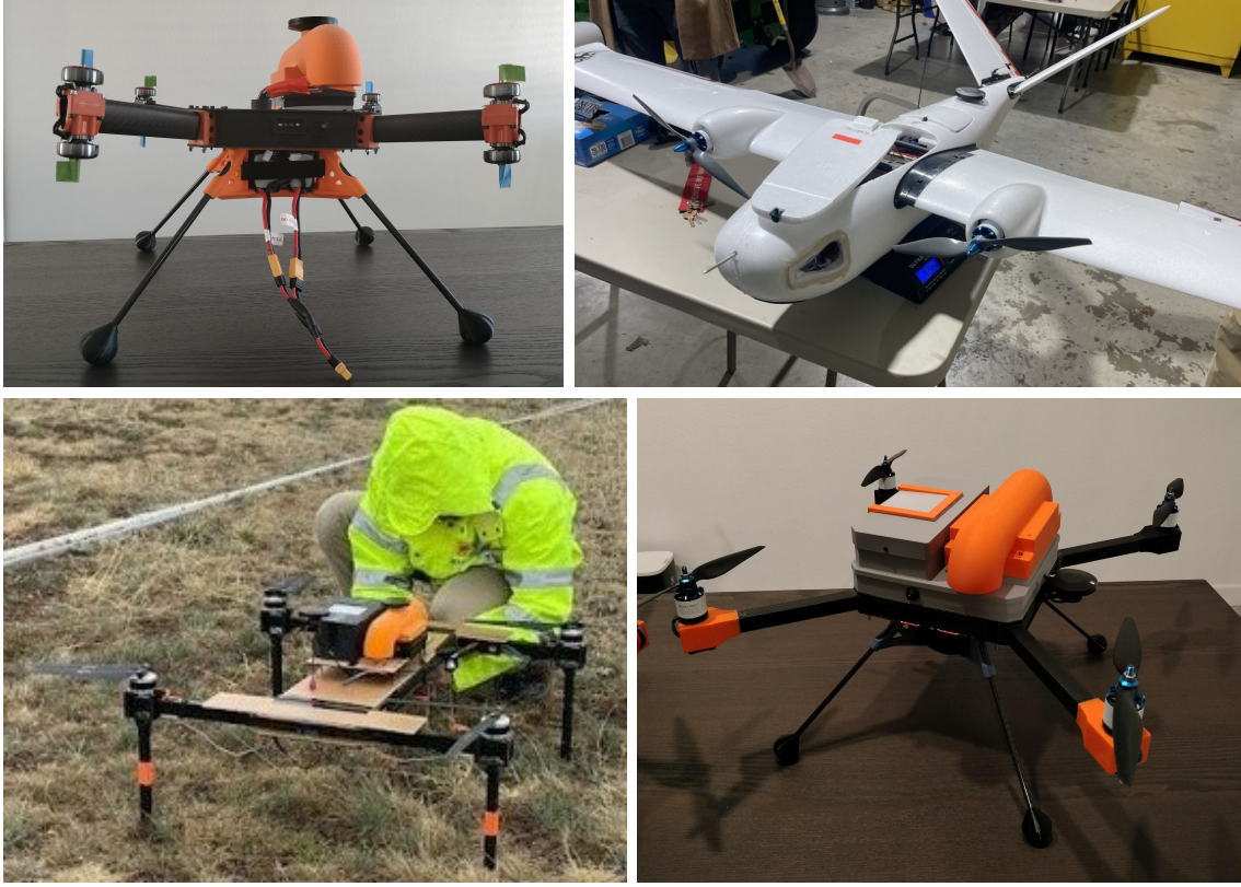
Figure 3.10: Examples of cross-platform use of the proposed WxUAS in-situ sensor hardware and software.
