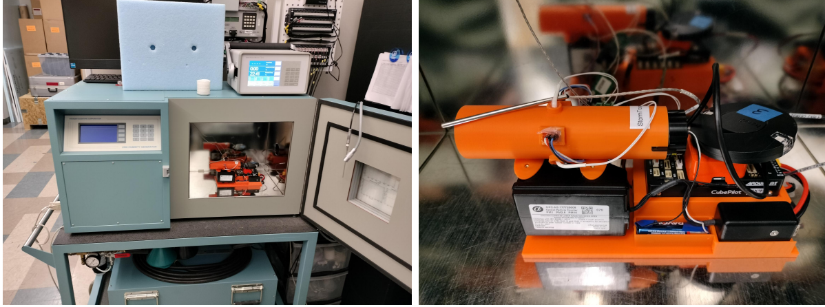
Figure 3.11: In-situ inner shield calibration at the Oklahoma Mesonet’s Calibration Laboratory. The left panel shows the Thunder Scientific 2500 benchtop humidity generator, and the right panel details the experimental setup inside the chamber’s test section.
