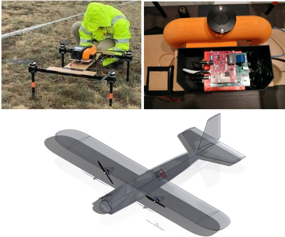
Figure 4.5: Illustration of cross-platform application of this chapter’s proposed remote measurement solution. Images on the top detail the integration into Oklahoma State University’s Skateboard, and the bottom image depicts a conceptual design for fixed-wing deployment.
