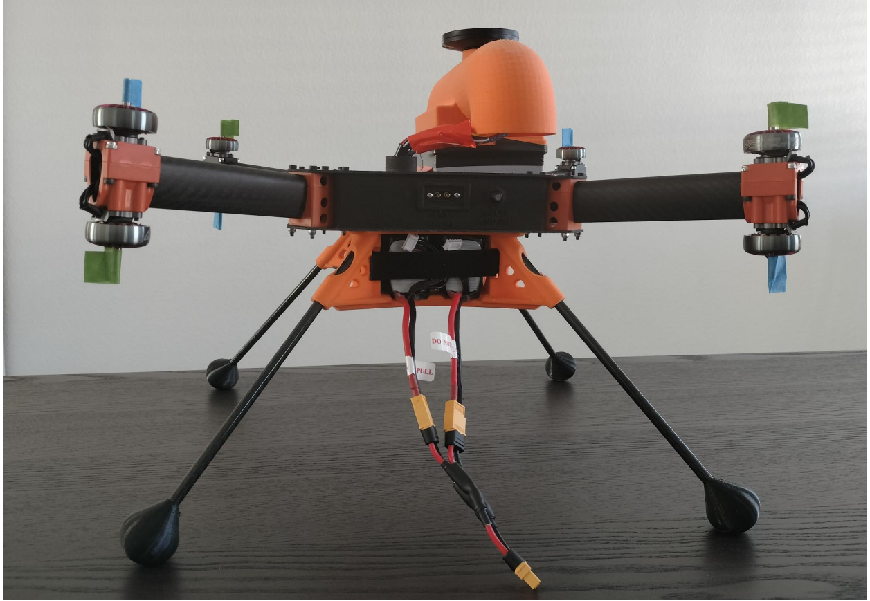
Figure 5.7: X-Frame co-axial quadcopter implementation of a partial version of this design for increased resiliency against icing.
