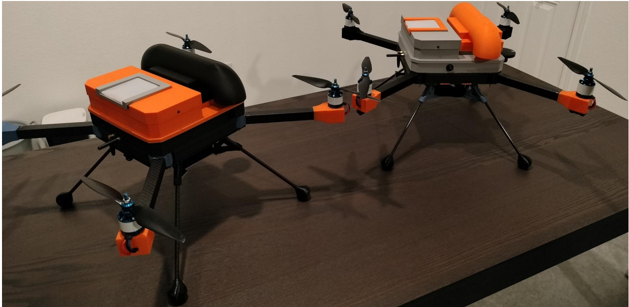
Figure 5.8: Two units of the StormTrooper winter precipitation WxUAS built for the MAI 2 S field campaign. This configuration represents the baseline for this dissertation’s proposed WxUAS aircraft design.
