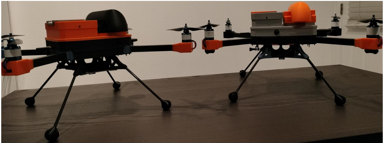
Figure E.4: Two units of this dissertation’s WxUAS aircraft design in the baseline configuration. These two units were purpose-built for the MAI 2 S field campaign.
