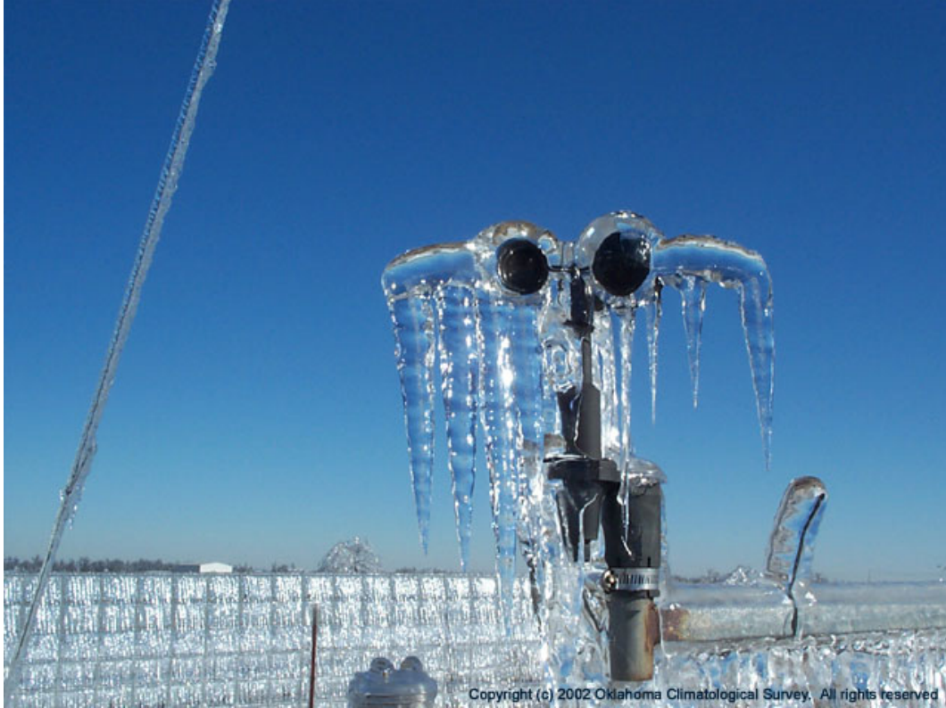
Figure 2.1: Example of environmental interference, a frozen cup anemometer at the Kingfisher Oklahoma Mesonet tower after the ice storm of January 28-30, 2002. Photo by Chris Fiebrich.
