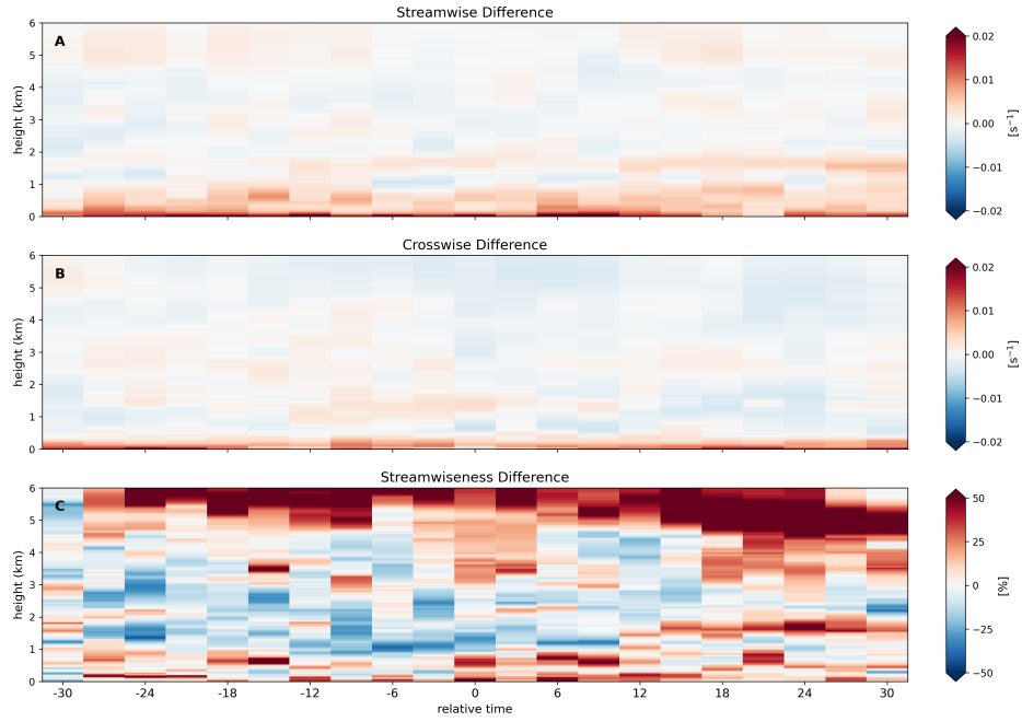
Figure 3.37: Differences in the streamwise (A) and crosswise (B) horizontal vorticity and streamwiseness (C) between tornadic and non-tornadic storm environments for the 0-6km layer.
