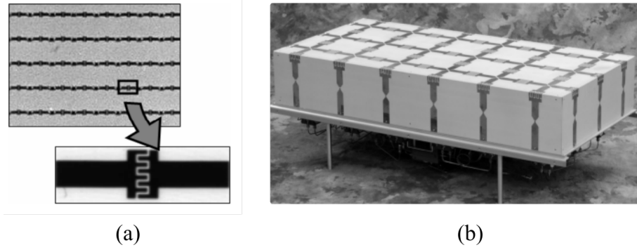
Figure 2.1: Tightly-Coupled Dipole Array having frequency range between 2-18 GHz (a) single-polarized (b) dual-polarized [32].
