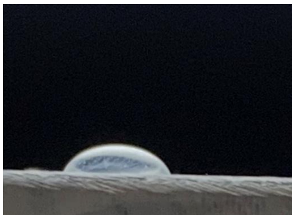
Figure 9: Water droplet on non-hydrophobic surface. The attachment angle on an aluminum surface is slightly less than 80^\circ
