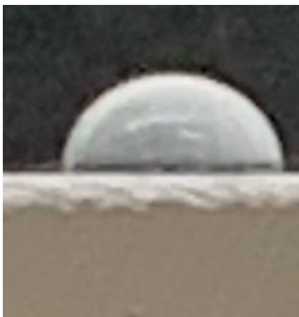
Figure 8: Water droplet on Adam's Graphene Ceramic Coating compound. The attachment angle on an aluminum surface is slightly greater than 90^\circ .
