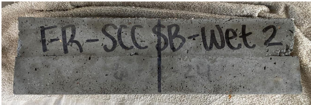
Figure 33: FR-SCC Composite Specimen after 307 Exposure Cycles
