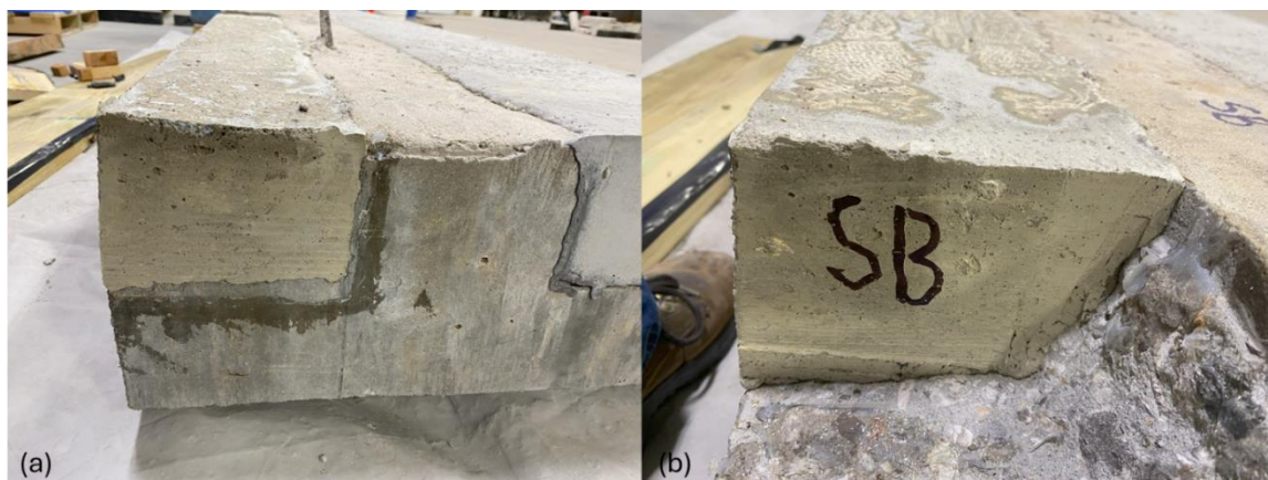
Figure 38: RS-SCC Interfaces on Large-Scale Repair Slab
