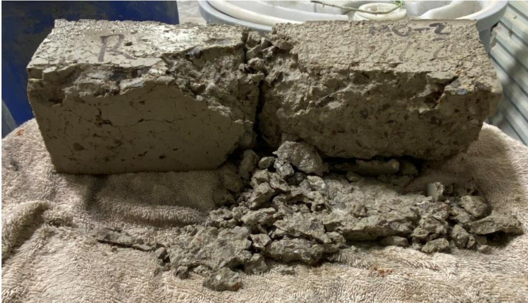
Figure 26: Deterioration of RS-SCCUA After Freeze-Thaw Exposure
