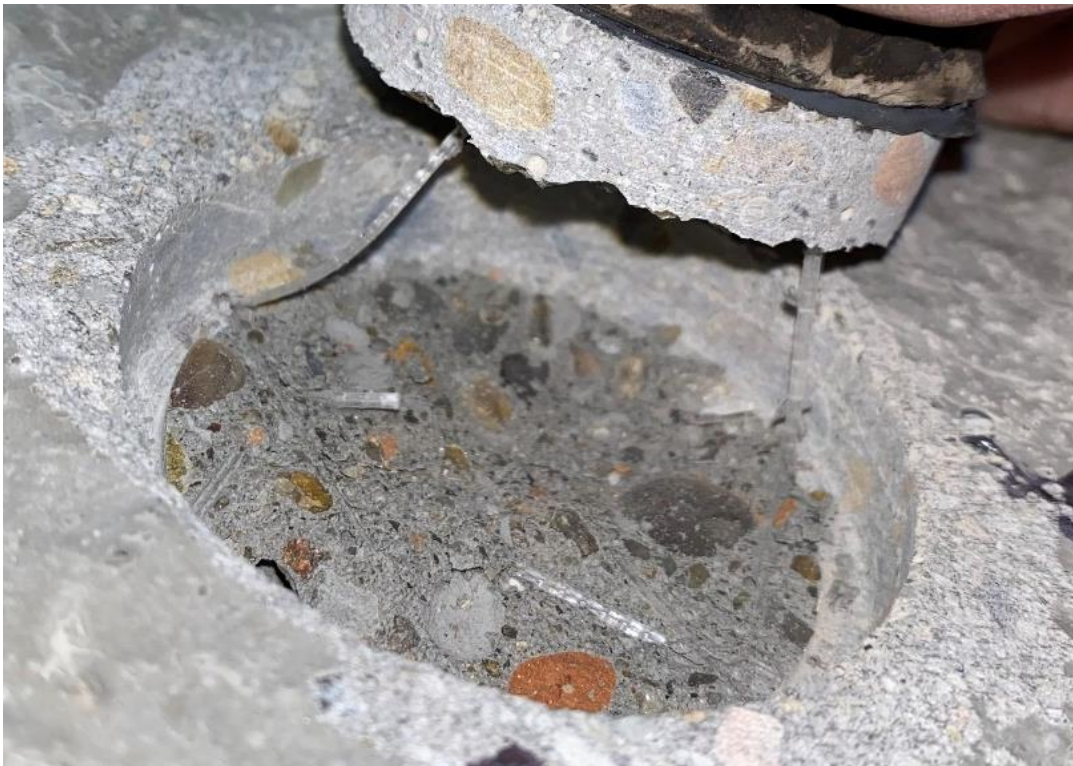
Figure 14: Polypropylene Fiber Bridging Failure Plane of Monolithic FR-SCC Pull-Off Specimen
