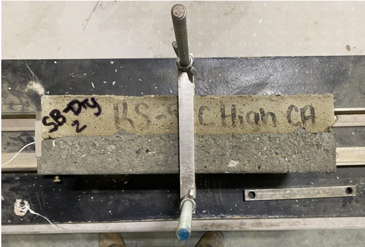
Figure 8: Specimen Orientation for Resonant Frequency Testing
