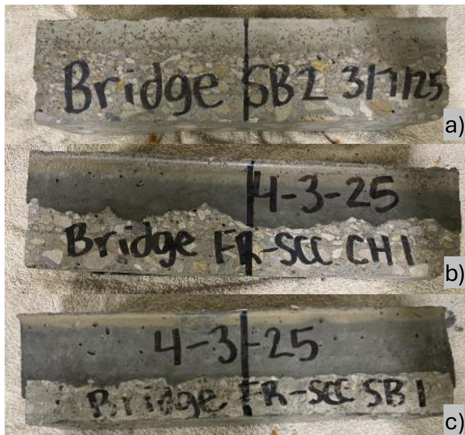
Figure 37: Bridge Deck Repair Specimens After Initial Exposure Period: RS-SCCHA-SB Specimen After 97 Cycles (a), FR-SCC-CH Specimen After 95 Cycles (b), and FR-SCC-SB Specimen after 95 Cycles (c)
