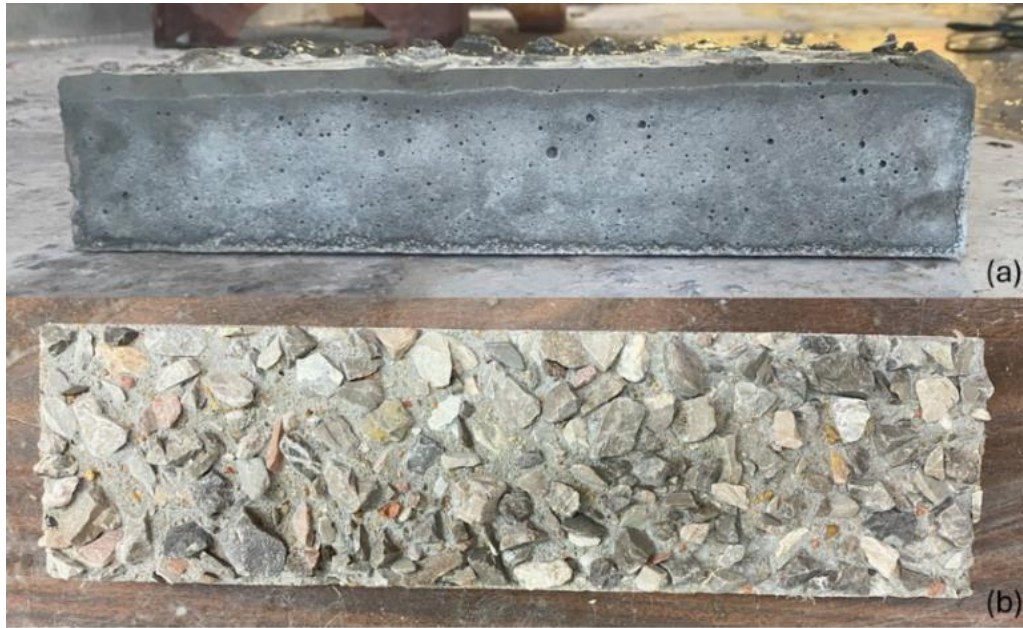
Figure 4: Visible Layer of Unset Paste (a) and Exposed Aggregate Finish (b)
