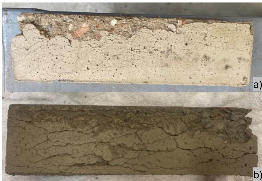
Figure 22: 7-Day (a) and 28-Day (b) Monolithic RS-SCC Specimens After Freeze-Thaw Exposure
