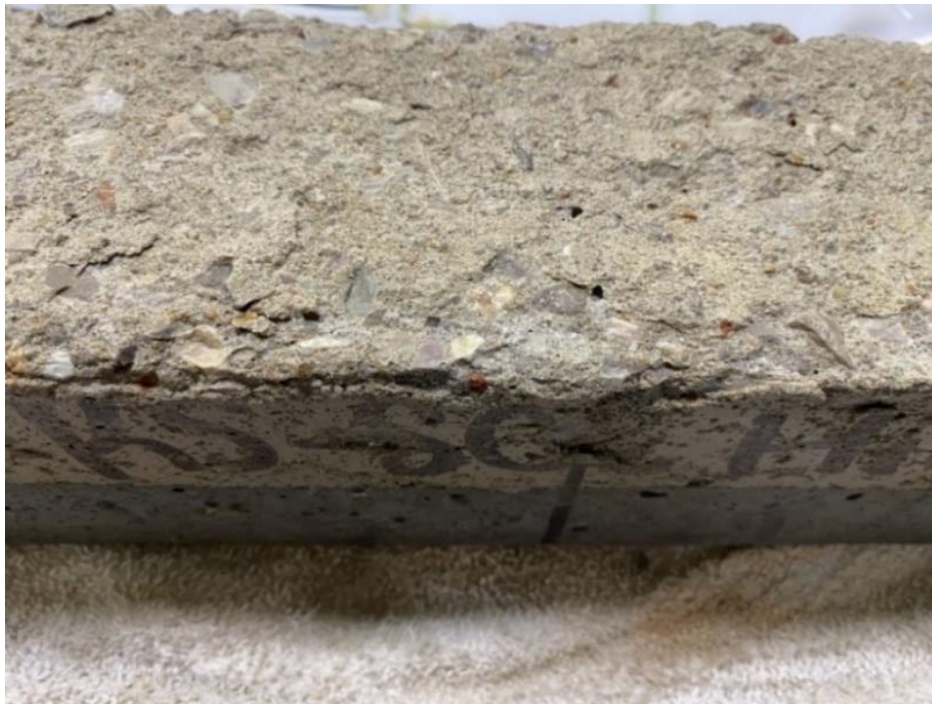
Figure 28: Crumbling of Edge and Surface of RS-SCCHA Specimen After Freeze-Thaw Exposure
