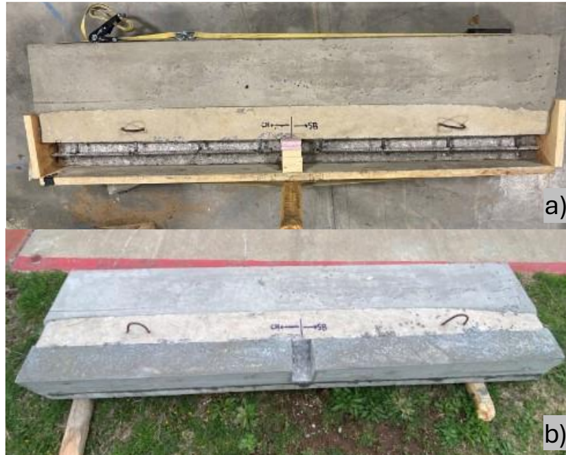
Figure 12: Large Scale Repair Slab Formwork (a) and Finished Specimen (b)
