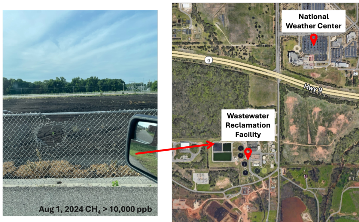
Figure 7.1 CH 4 Concentration measurement at the City of Norman Wastewater Reclamation Facility. The right panel shows the City of Norman Wastewater Reclamation Facility as seen from Google Earth, with the National Weather Center located just across Highway 9. The left panel captures the solid sedimentation pond at the facility, where methane concentrations exceeding 10,000 ppb were measured downwind of the pond on August 1, 2024.
