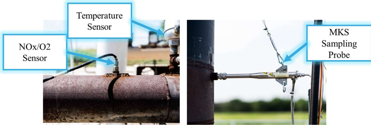
Figure 11: Temperature, NOx/O2, and MKS Sampling Line on the AJAX Engines
