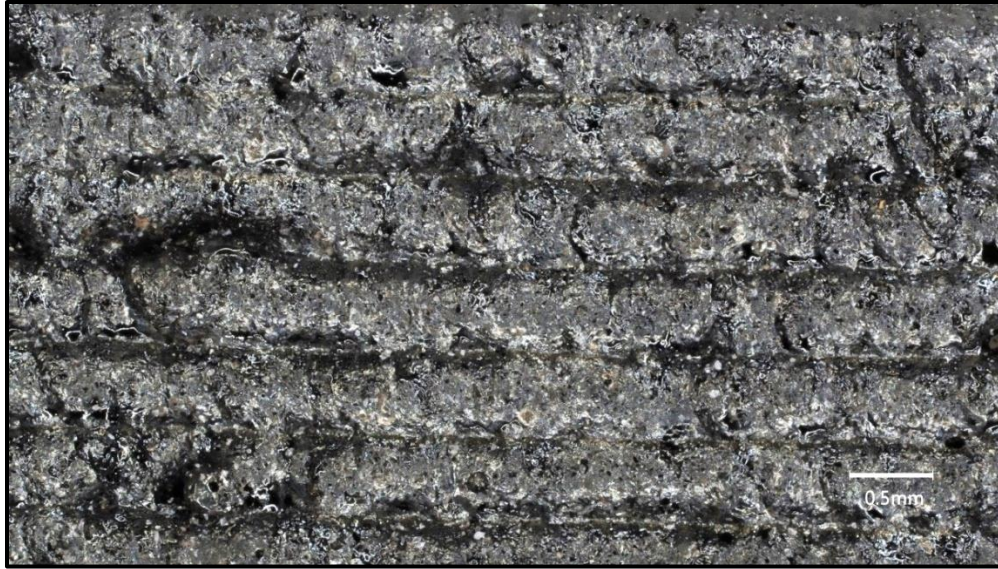
Figure 34: Optical Image of General Parallel Bonding in SiC Square Specimen
