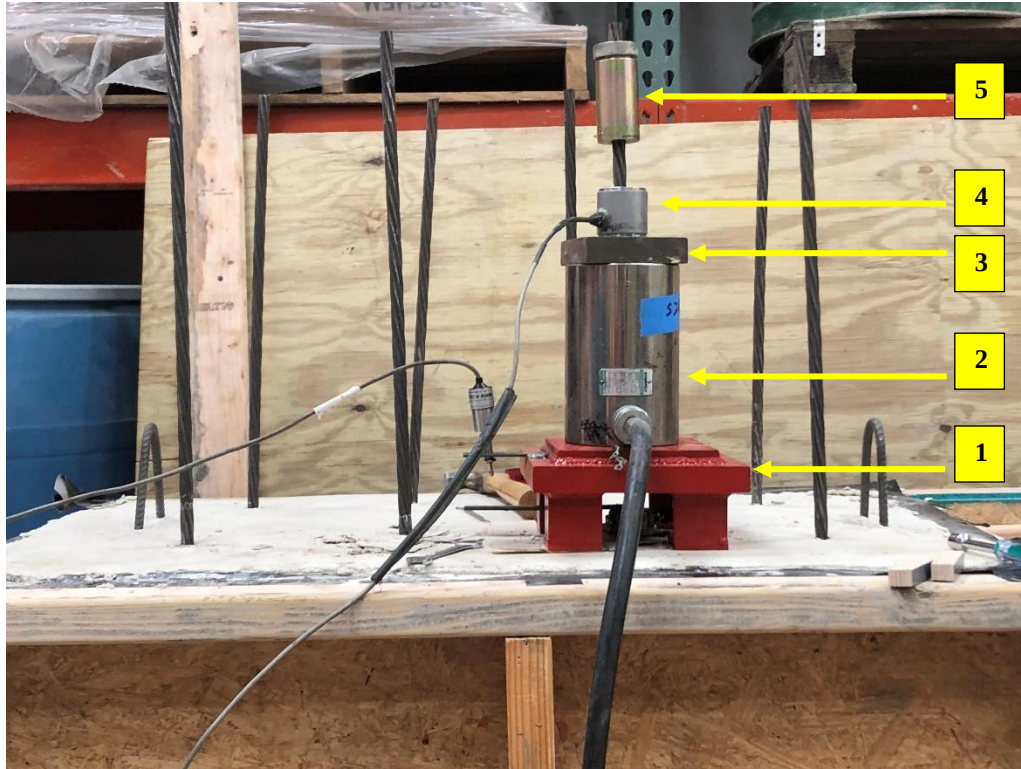
Figure 62: Testing setup for direct strand pullout with load and slip measurement used for the LBPT
