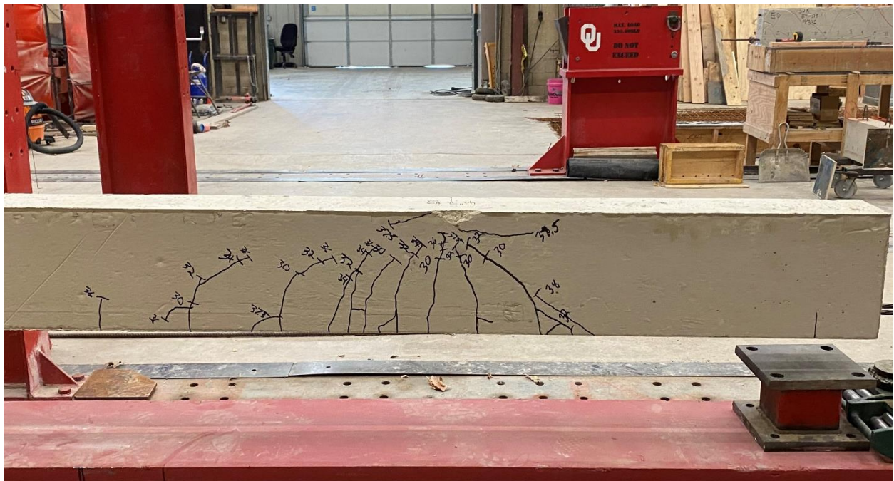
Figure 104: Trial beam B2 dead end after failure showing flexural cracking and top crushing
