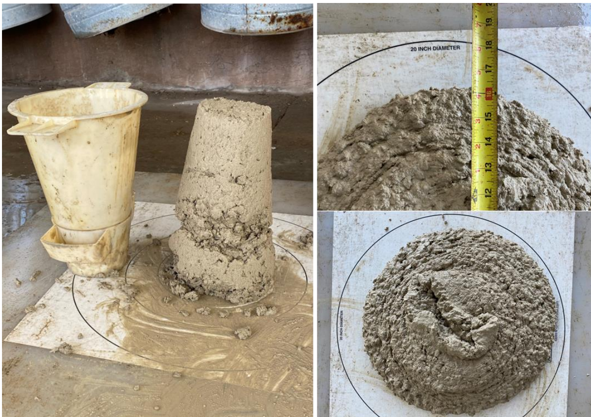
Figure 92: 20-minute slump comparisons for mixes FR1 (conventional slump, left – 0 in.) and FR2 (slump flow, right – 16 in.)
