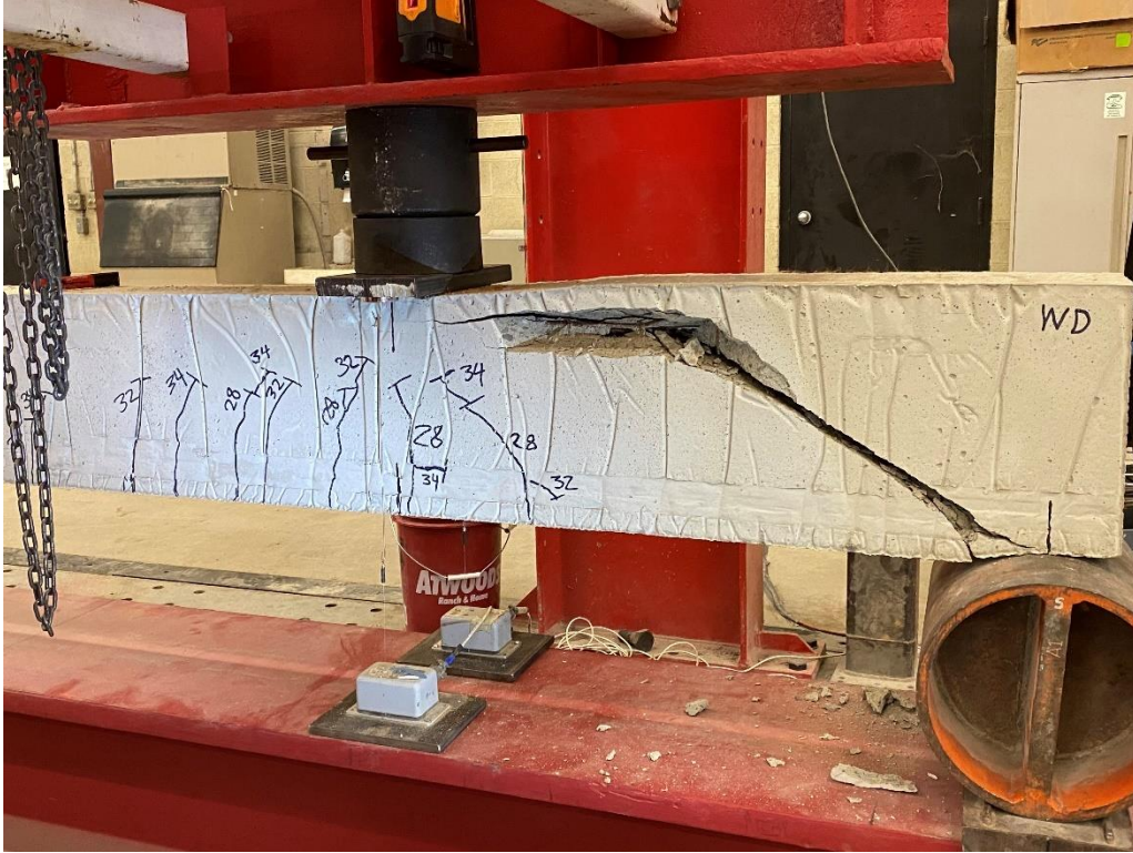
Figure 116: Cracking pattern at failure for B7-3DV with 3 ft embedment (dead end)
