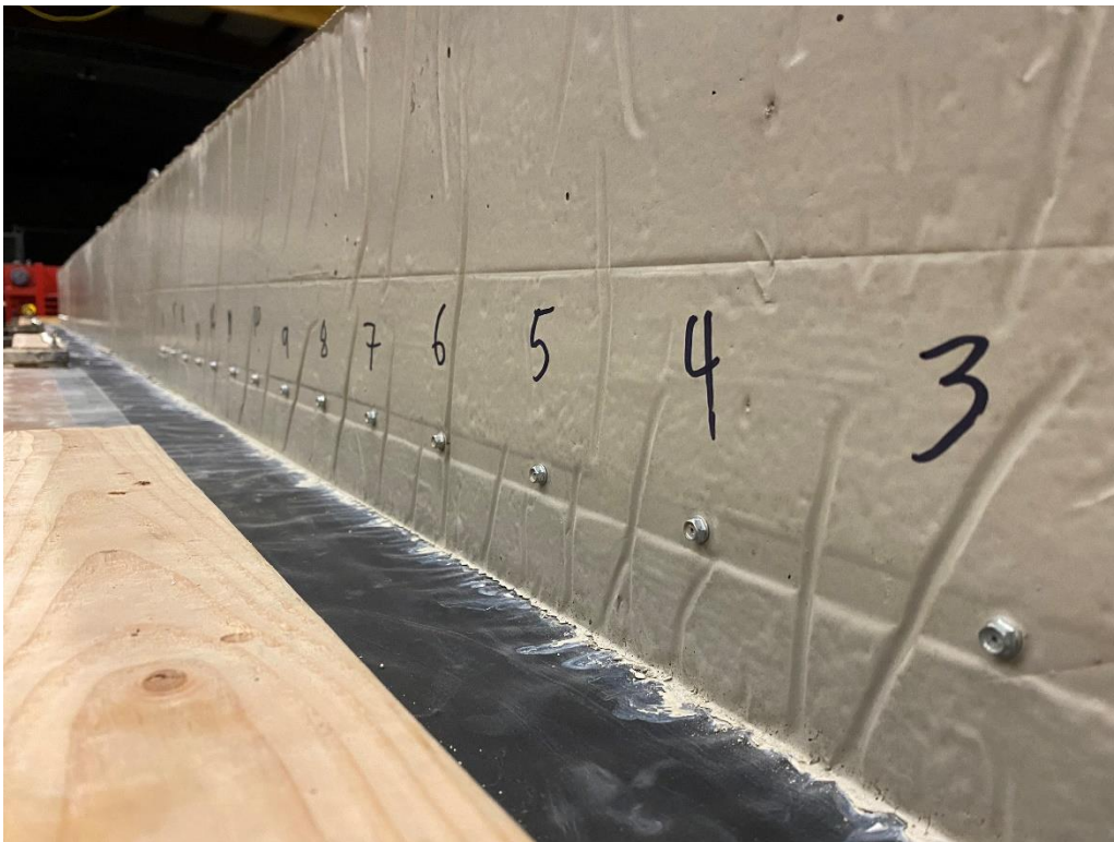
Figure 144: Longitudinal distribution of DEMEC instrumentation for surface strain profile measurement
