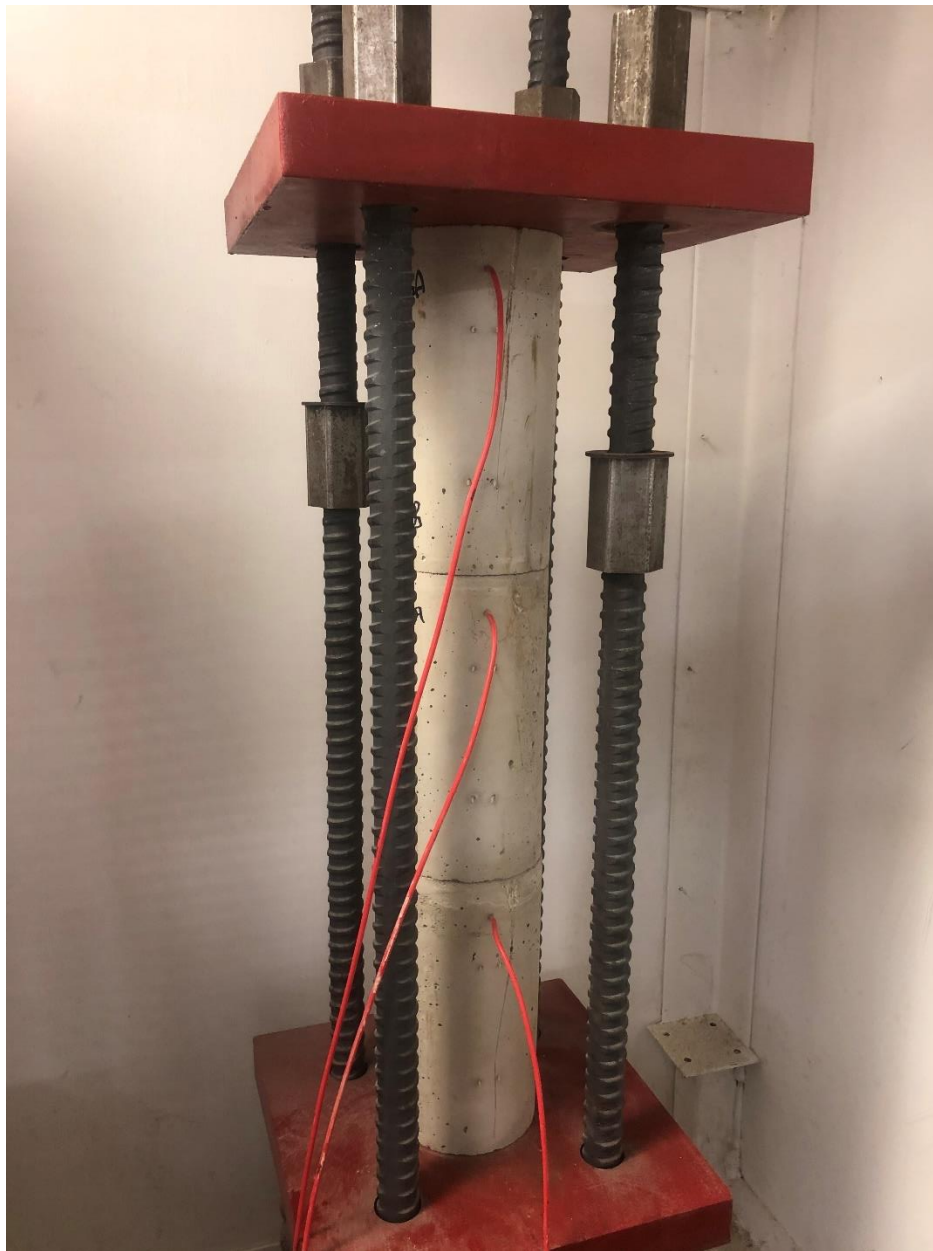
Figure 45: Creep specimens in final configuration, after load application, with instrumentation set and loading apparatus removed
