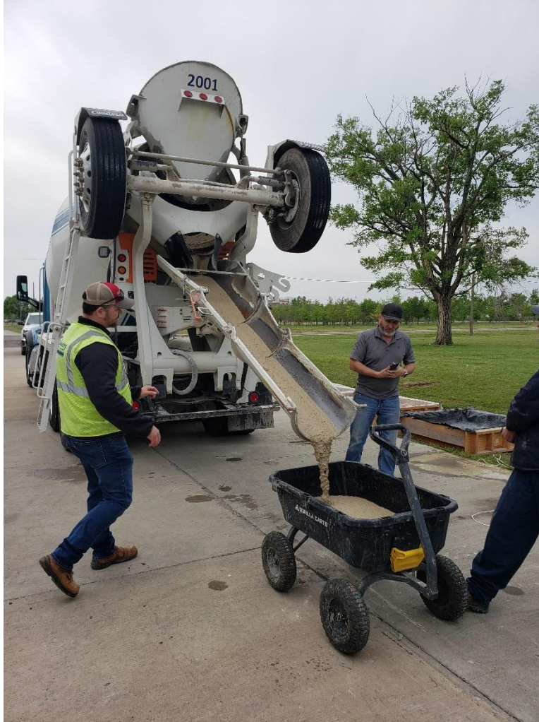
Figure 68: Dispensing small portion of LBPT mix to measure the slump flow
