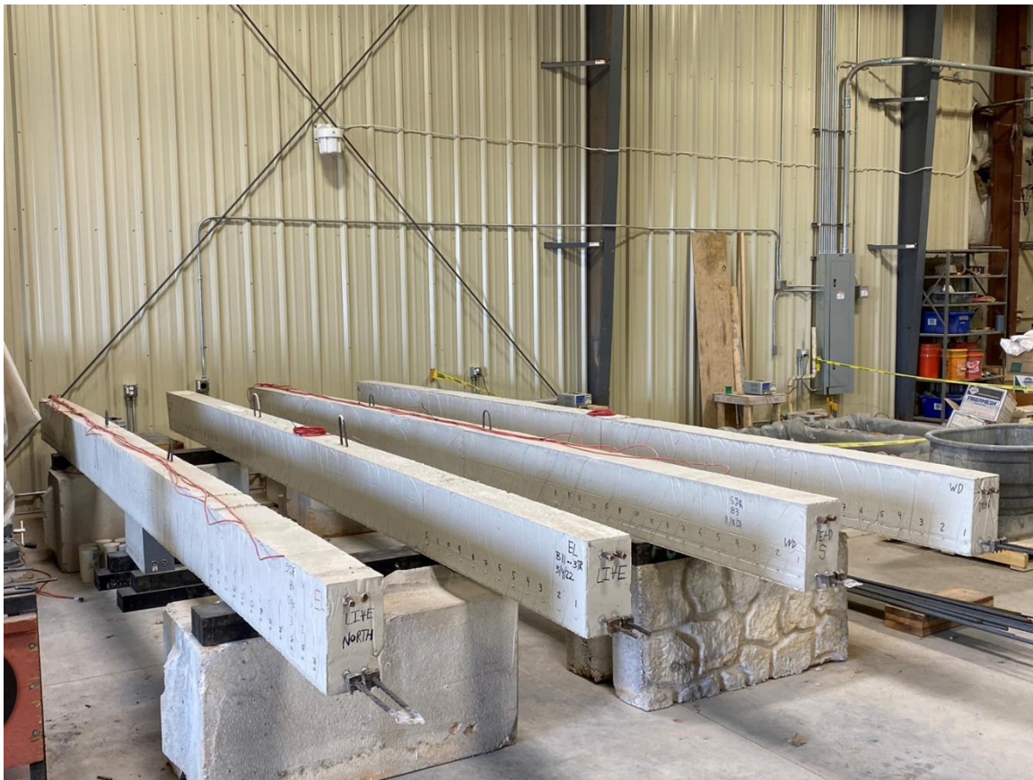
Figure 152: Beams in storage for long-term prestress loss measurement in Fears Lab high bay
