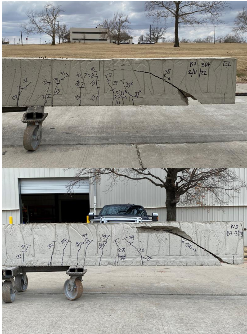
Figure 117: Comparison of cracking pattern at failure for B7-3DV with 3 ft embedment - live end (top) and dead end (bottom)
