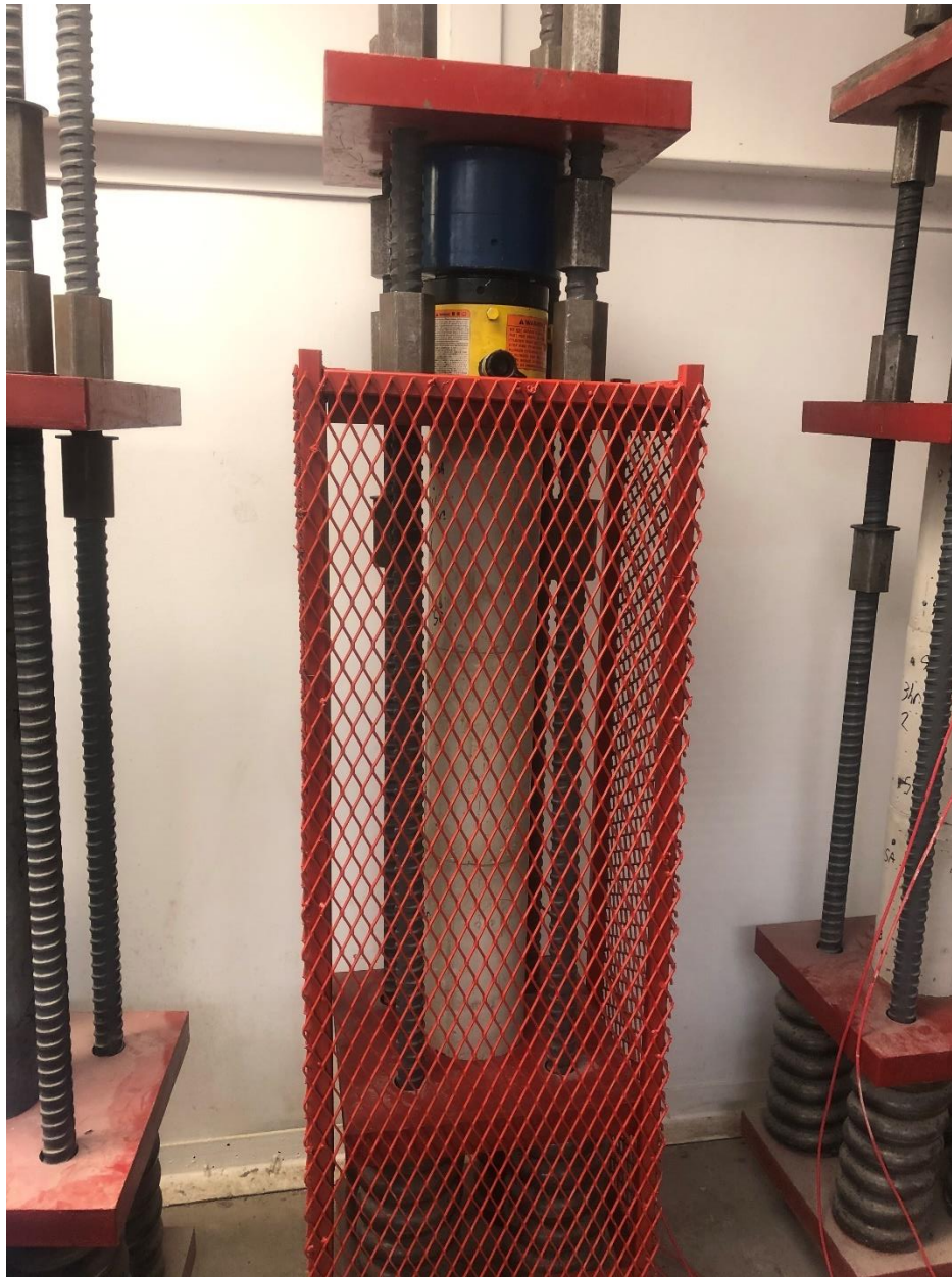
Figure 44: Creep frame with safety cage for stressing creep specimen in place
