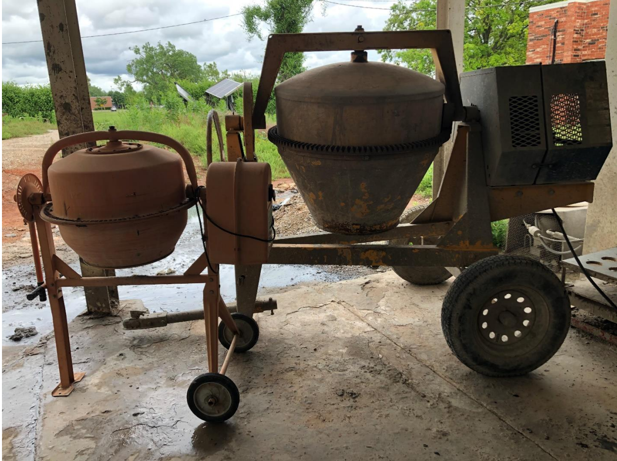
Figure 13: Small 1 ft 3 capacity rotating drum mixer (left) and medium 6 ft 3 capacity rotating drum mixer (right) – [listed capacities are maximum mix volumes not rated capacities]
