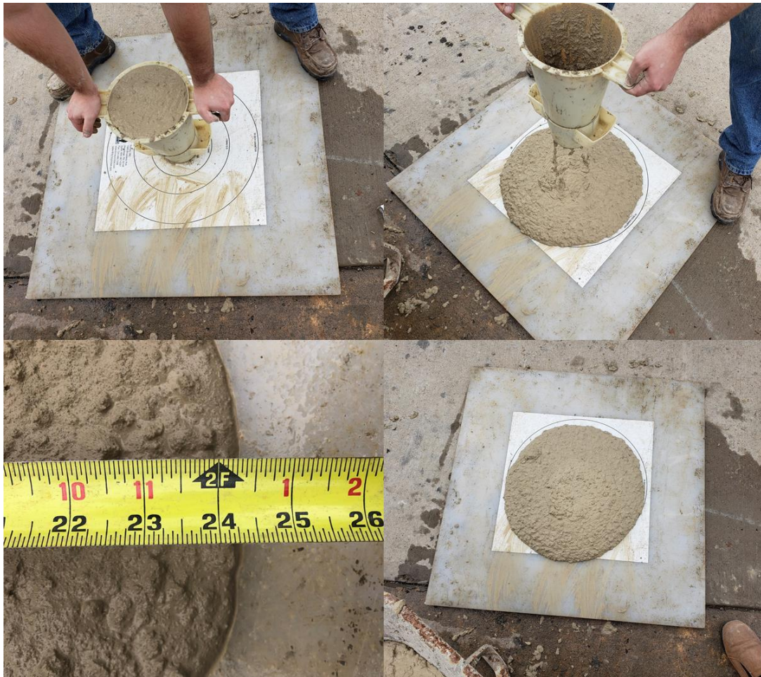
Figure 69: Slump flow measurement for full-scale LBPT pour (clockwise from top left)
