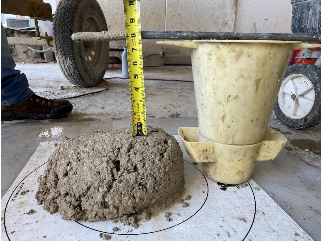
Figure 95: Conventional slump test of FR4 at 75 minutes (7.5 in.)
