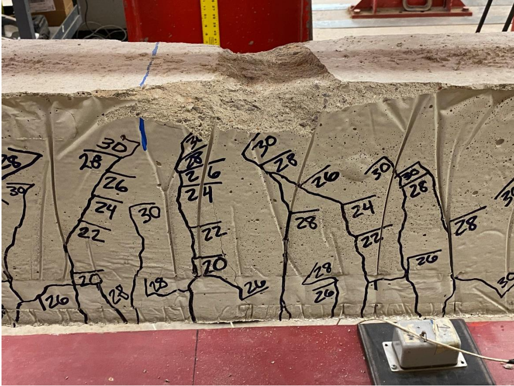
Figure 127: Compression block crushing and flexural cracking in B15-24DV (dead end)
