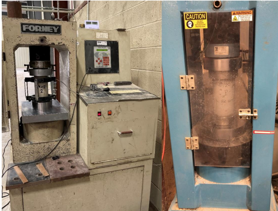
Figure 28: MOE test on Forney 1 (left) with compression test on Forney 2 (right)
