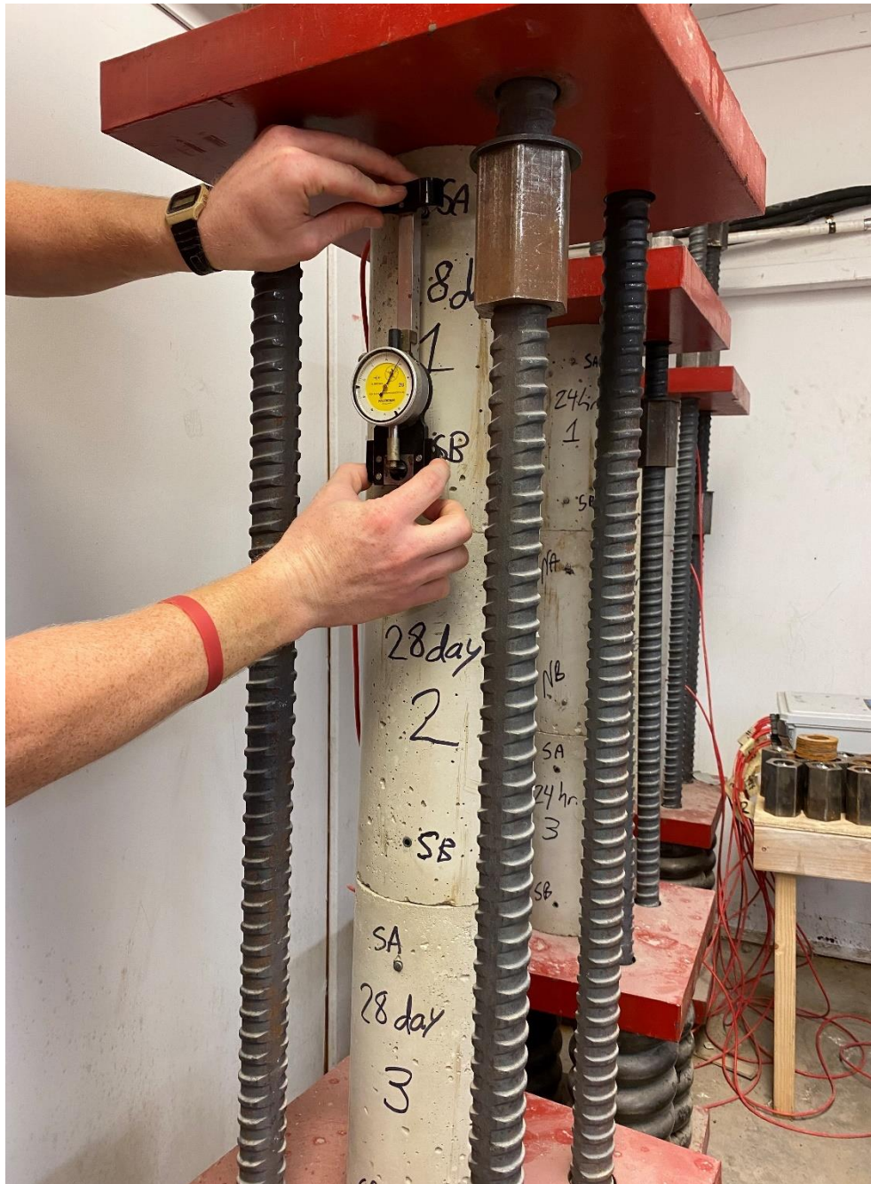
Figure 46: DEMEC gage being used to take creep strain measurements
