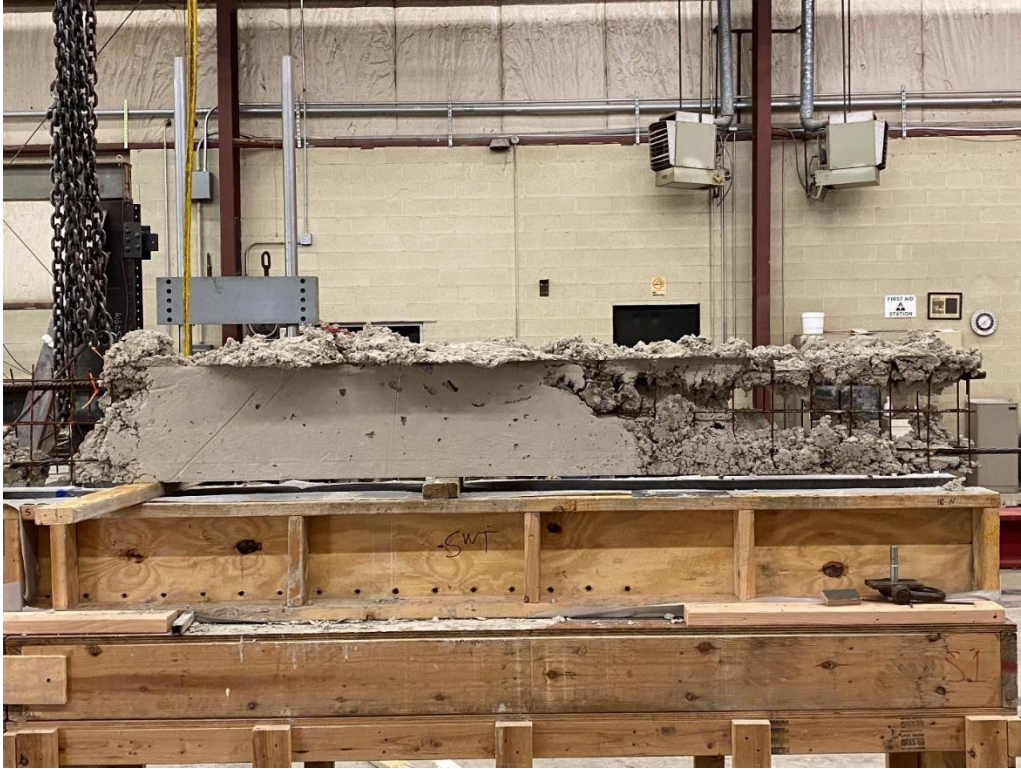
Figure 90: Profile view of trial beam B1 after formwork removal
