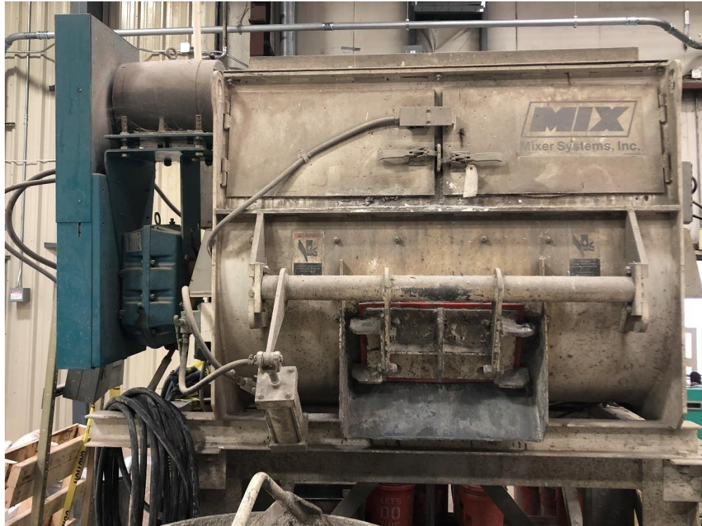
Figure 58: Praschak®/MIX Mixer Systems® 21 ft 3 horizontal shaft concrete mixer at Fears Lab (model no. 21 DD RH)
