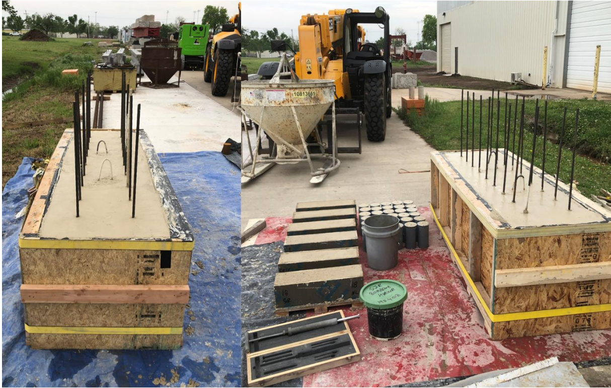
Figure 71: Completed LBPT specimen (left) with MOR beams, compressive cylinders, and setting time test in progress, covered with green lid (right)
