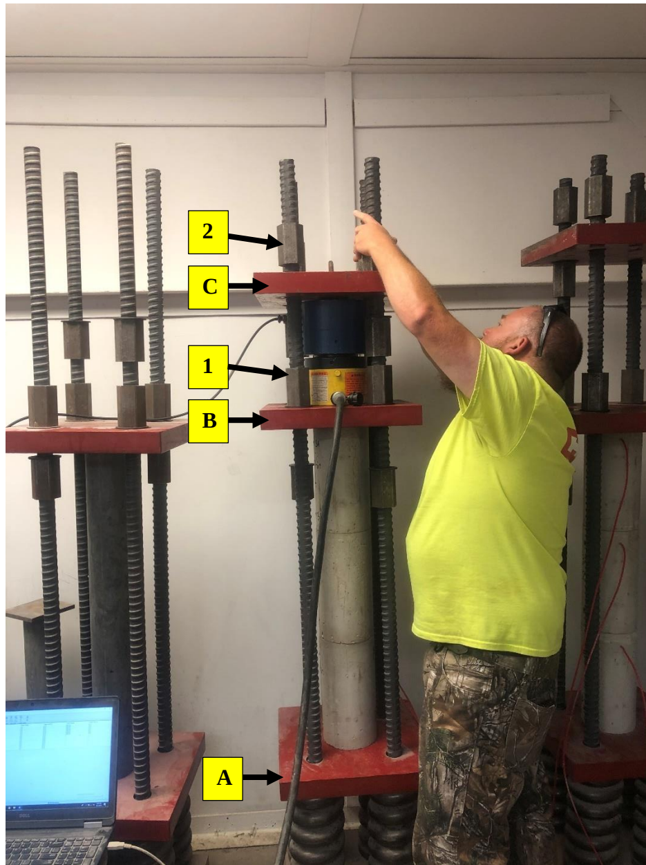
Figure 42: Setting reaction plates to load creep specimens
