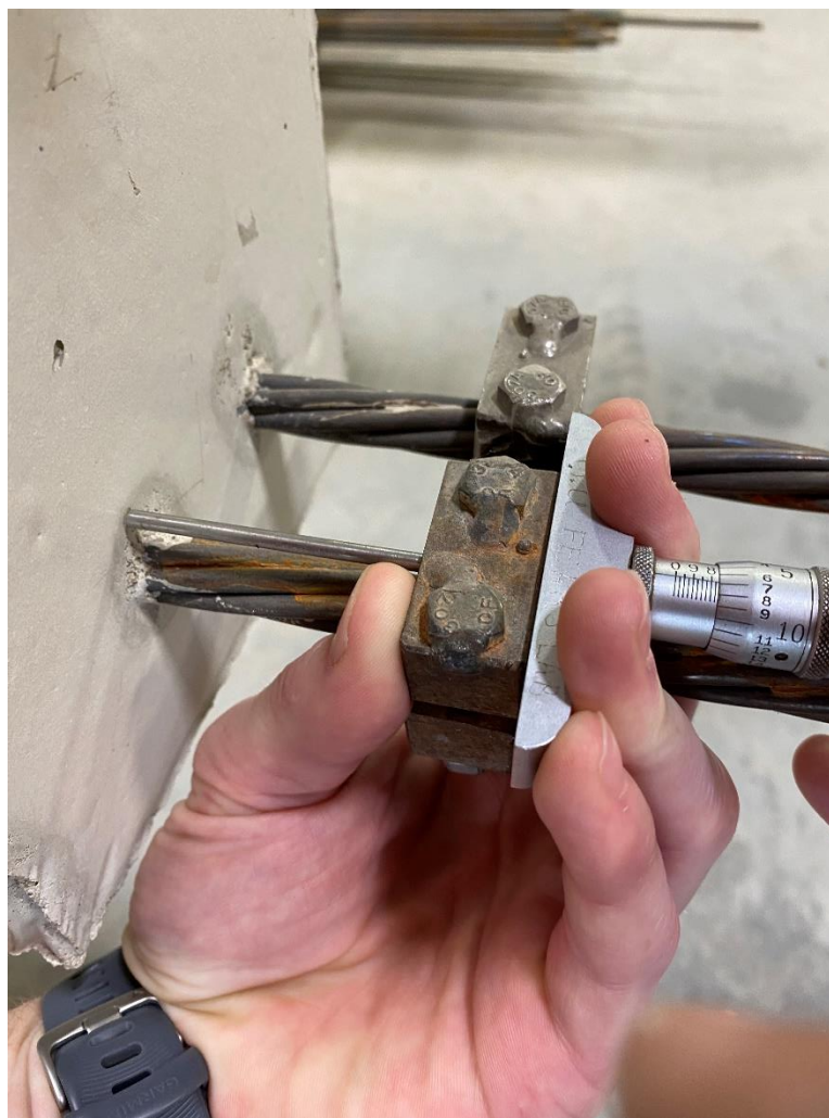
Figure 146: Typical strand draw-in measurement using a depth micrometer for TR series beam
