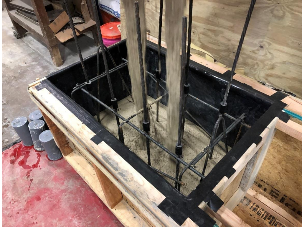
Figure 60: RS-SCC filling half-scale LBPT specimen formwork
