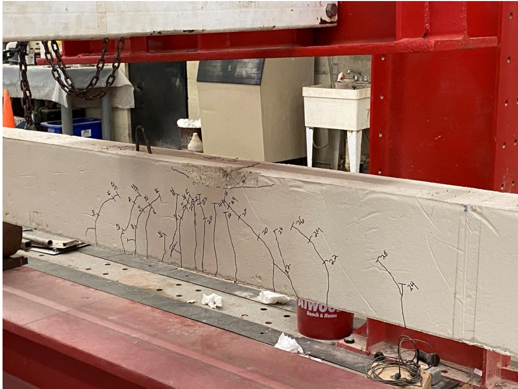
Figure 105: Trial beam B2 live end after failure showing flexural cracking and top crushing
