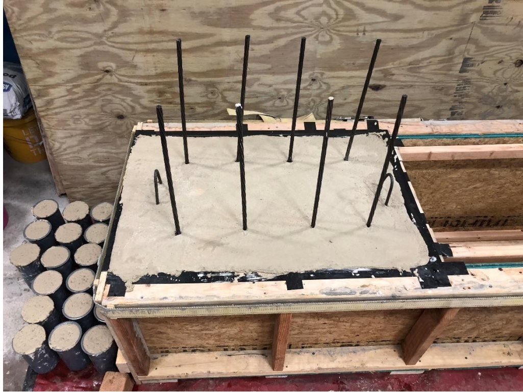
Figure 61: Half-scale LBPT specimen and compressive strength cylinders after casting
