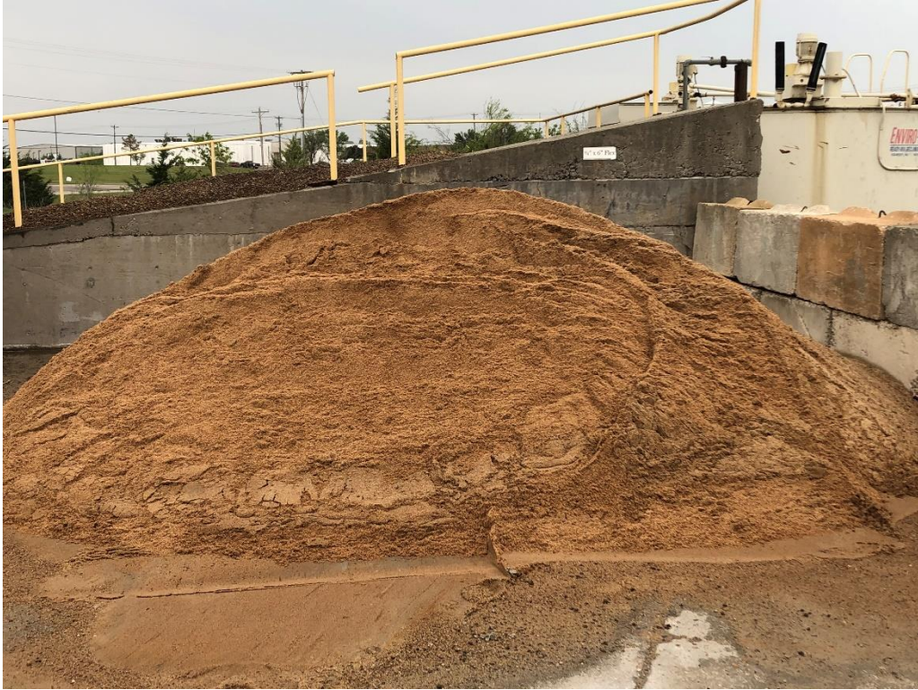
Figure 64: ASTM C33 fine aggregate (Dover sand) storage at Schwarz Ready Mix facility
