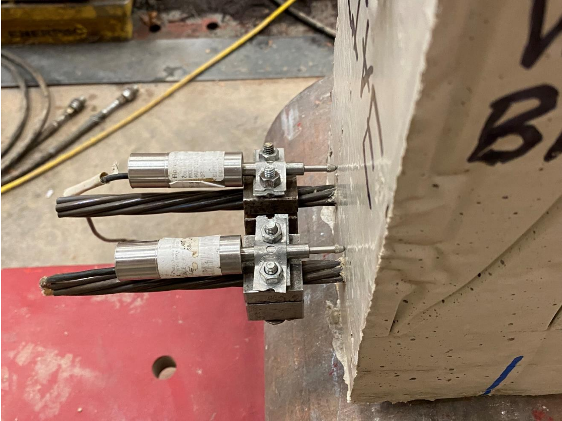
Figure 102: LVDT's mounted to strands with block clamps to measure strand slip
