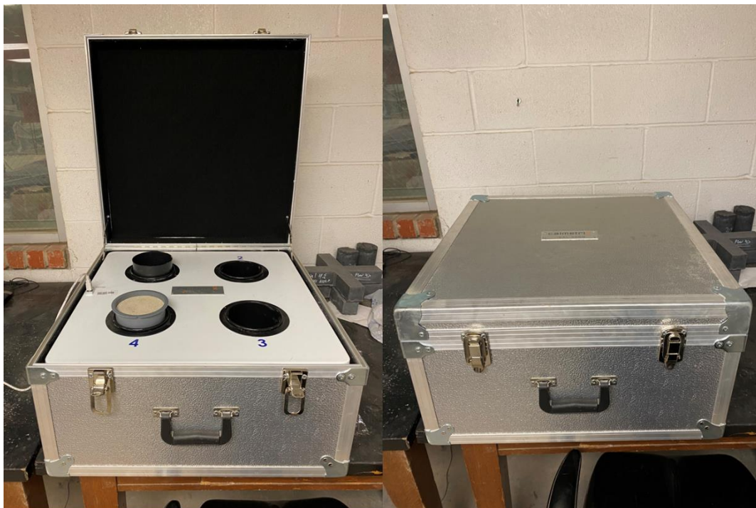
Figure 15: Calmetrix® Semi-Adiabatic Calorimeter
