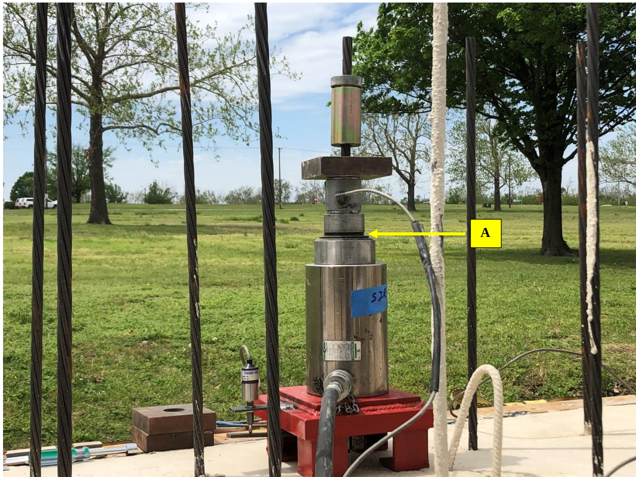
Figure 72: Hydraulic ram, load cell, and LVDT for strand pullout measurements
