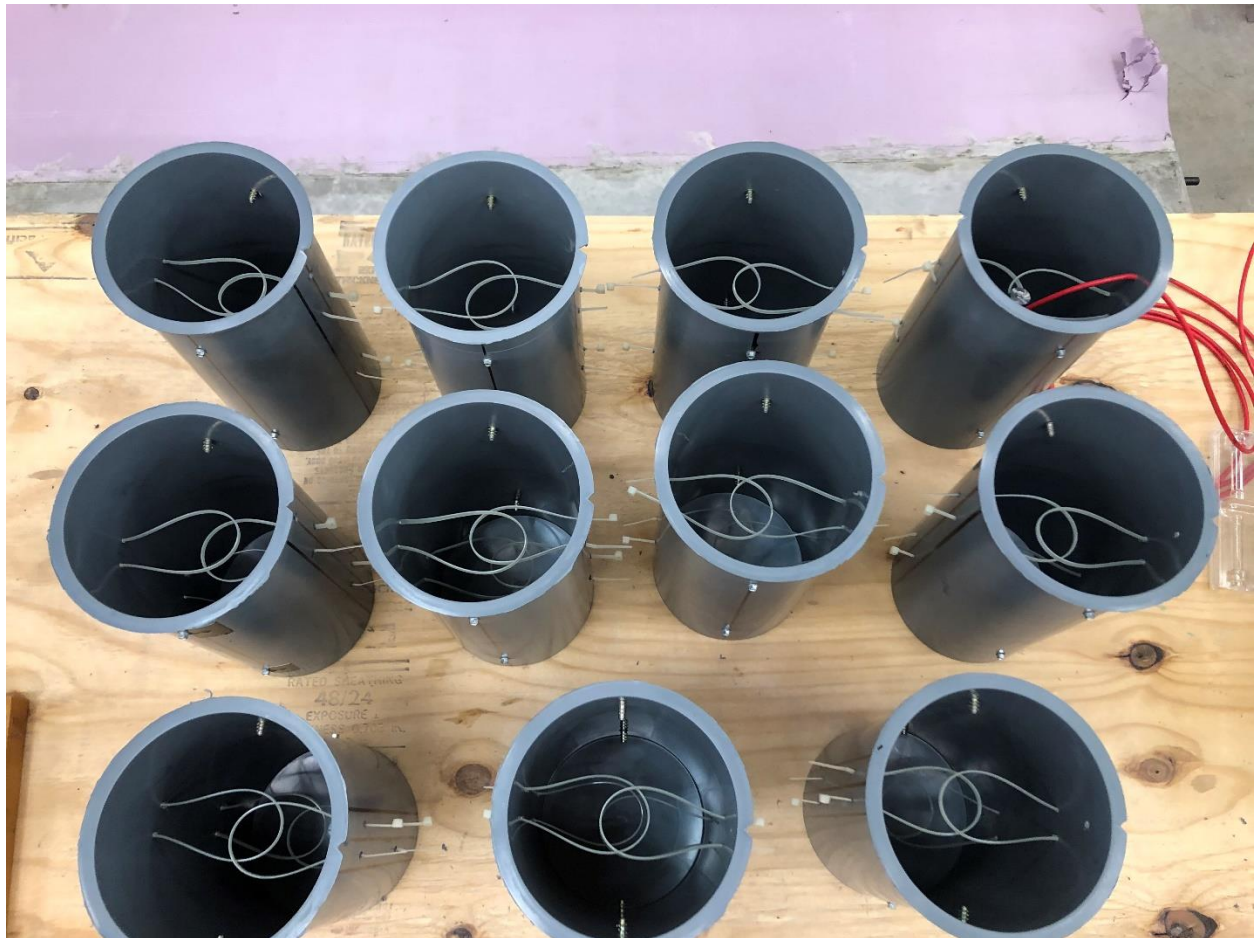
Figure 39: Creep specimen molds prepared for placement of the VWSG
