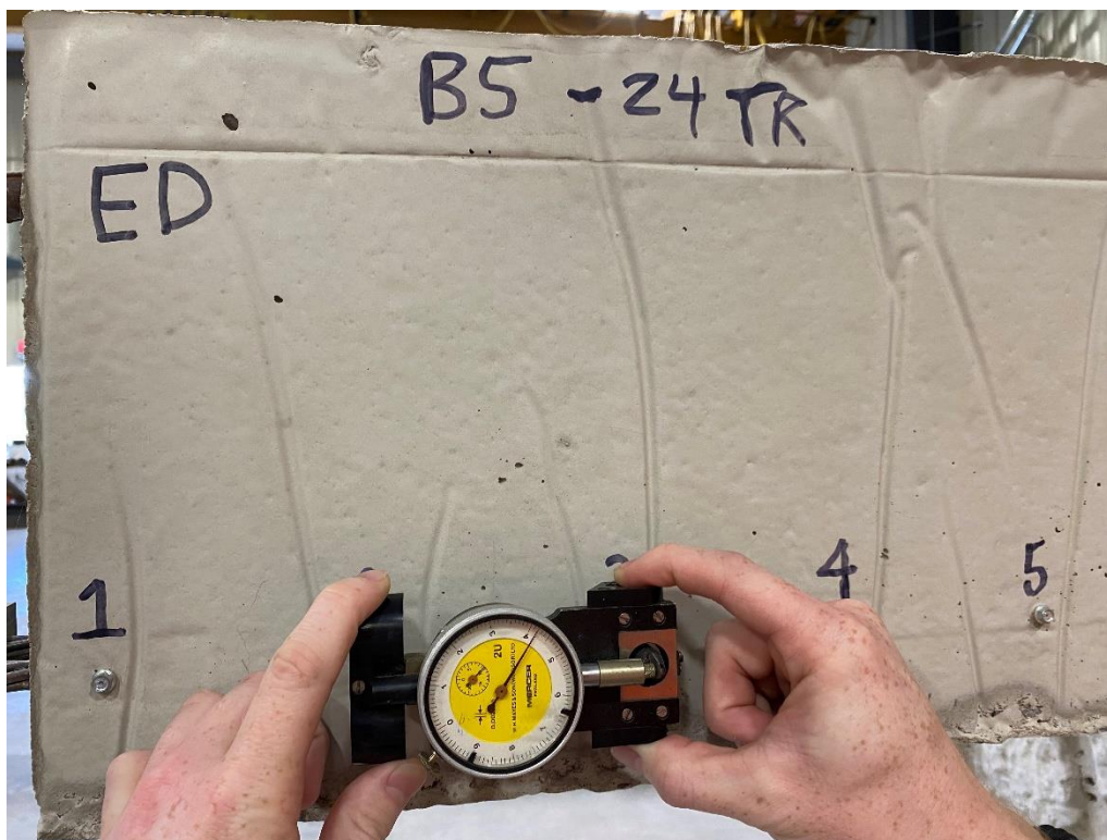
Figure 145: Typical DEMEC strain gage measurement for TR series beam
