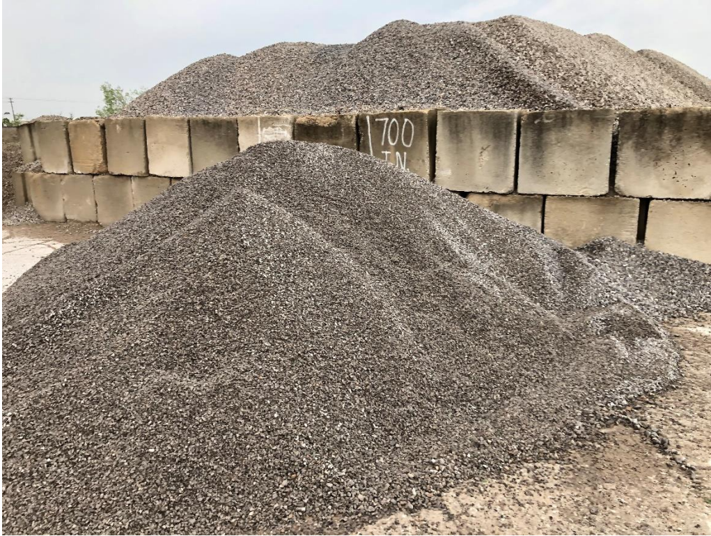
Figure 65: Dolese 5/8" #3 cover coarse aggregate storage at Schwarz Ready Mix facility
