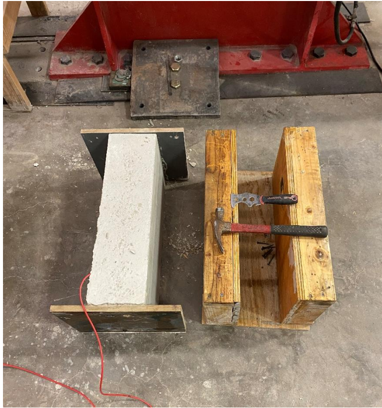
Figure 156: Non-prestressed companion beam for shrinkage measurements
