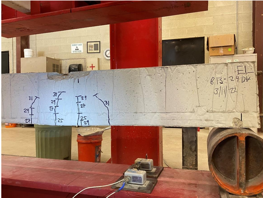
Figure 132: Cracking pattern at failure for B13-24DV with 3 ft embedment (live end)
