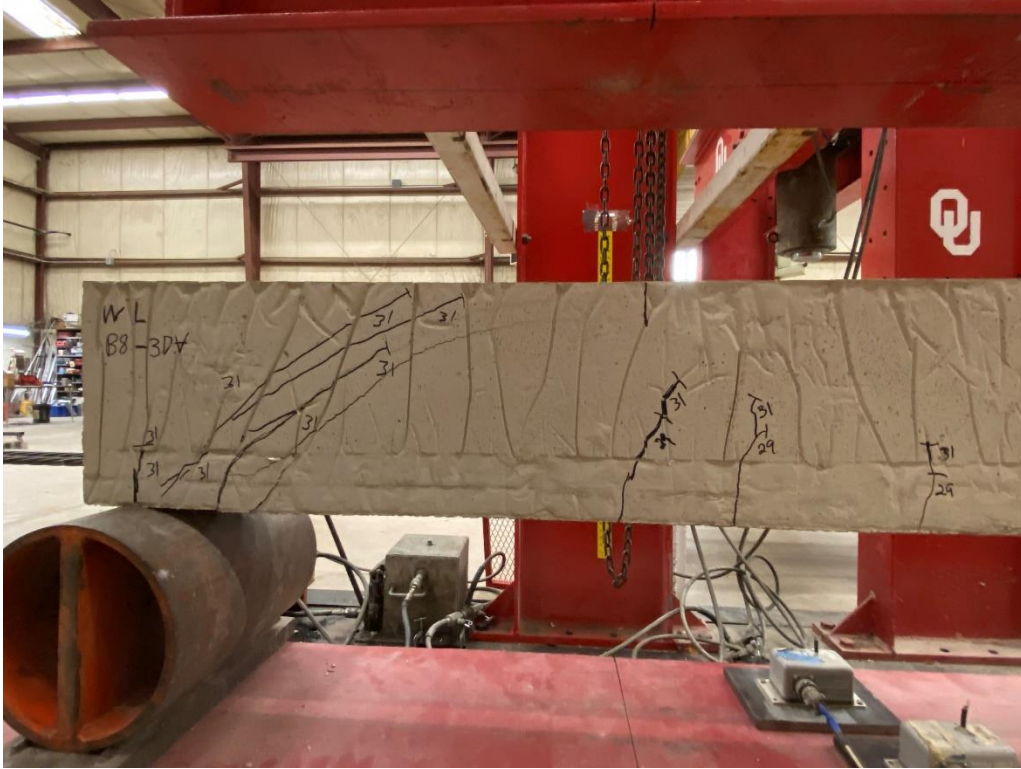
Figure 120: Cracking pattern at failure for B8-3DV with 2.5 ft embedment (live end)
