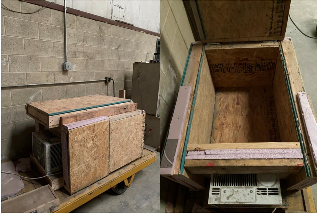
Figure 14: Insulated container used for conditioning aggregates for setting time mixes
