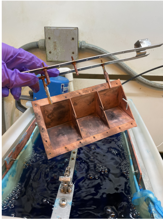
Figure 6.13: An image of the electroplating rack and tank
