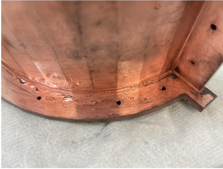
Figure 6.12: An example image of delamination of copper during the electroless plating process
