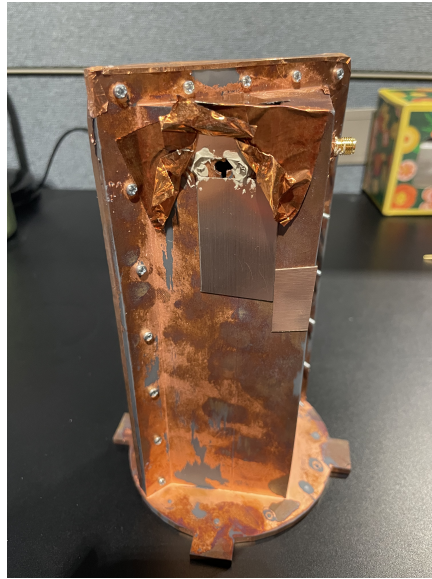
Figure 6.22: An image of the first filter prototype with the copper tape covered crack visible
