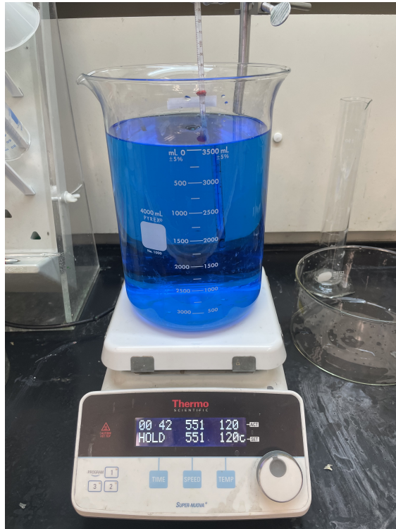
Figure 6.10: An image of the electroless plating bath used to deposit the copper seed layer
