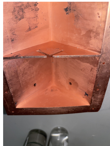
Figure 6.14: Example images of the (a) outside of a resin print, and (b) inside of the piece after the first electroplating cycle
