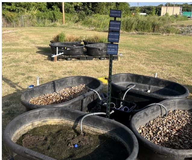
Figure 6 : Solar-powered aerator installation for one FWS, one OWC, and two SSF mesocosms.
