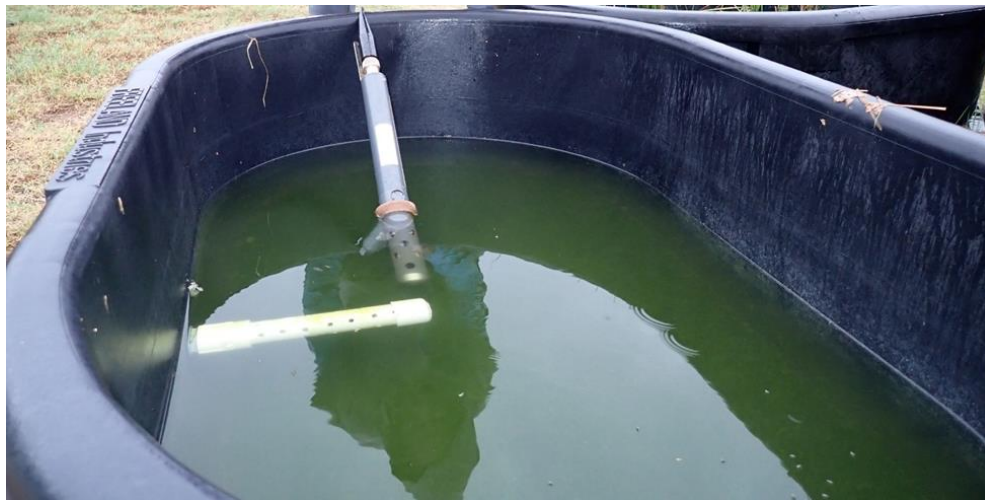
Figure 11 : OWC mesocosm with green algae and multiparameter data sonde on final day of experimentation.
