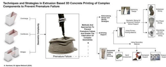
Figure 2: Extrusion-Based 3D Printing Construction method (Kamhawi & Aghaei Meibodi, 2024)
