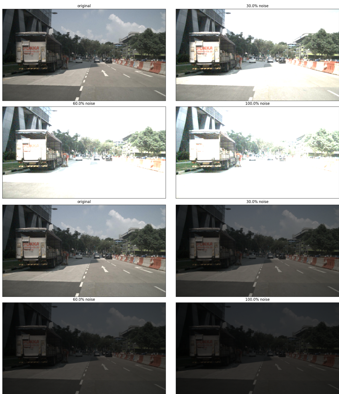
Figure 3.2: Overexposure (top) and underexposure (bottom) degradations at 0% (original), 30%, 60%, and 100% (max) distortion levels
