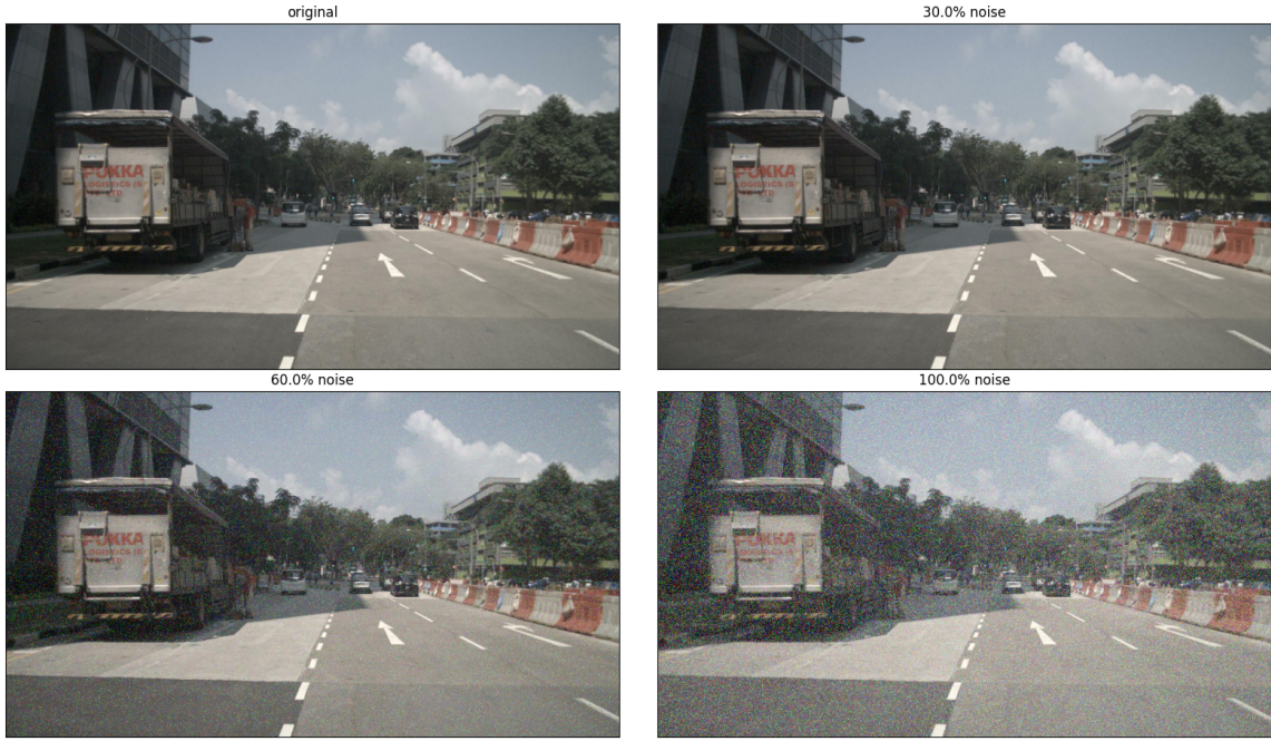
Figure 3.3: Normally distributed additive noise degradation at 0% (original), 30%, 60%, and 100% (max) distortion levels
