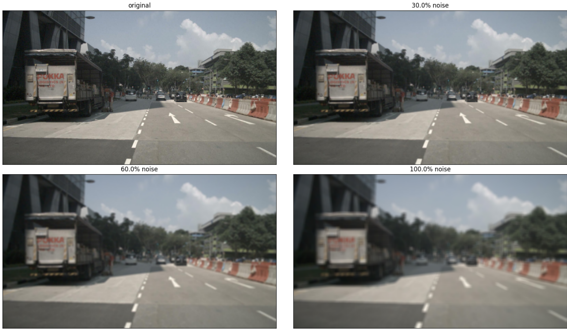
Figure 3.1: Blur effect at 0% (original), 30%, 60%, and 100% (max) distortion levels
