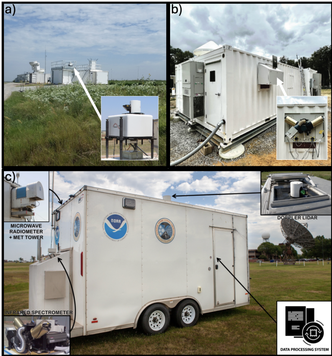
Figure 2.1: Pictures of ARM-CF's lidar (Fig. 2.1a), ARM-CF's AERI (Fig. 2.1b), and the CLAMPS2 platform (Fig. 2.1c), along with zoom-in pictures of each instrument. Though only the CLAMPS2 trailer is shown here, CLAMPS1 mirrors its setup. The Fig. 2.1a, 2.1b, and 2.1c pictures were provided by Corydon Ireland at https://ar.r.science.energy.gov/news/program-news/post/10247 and Gero and Hackel (2025), respectively, and the CLAMPS2 pictures were provided by NSSL at https://apps.nssl.noaa.gov/CLAMPS/ , respectively.
