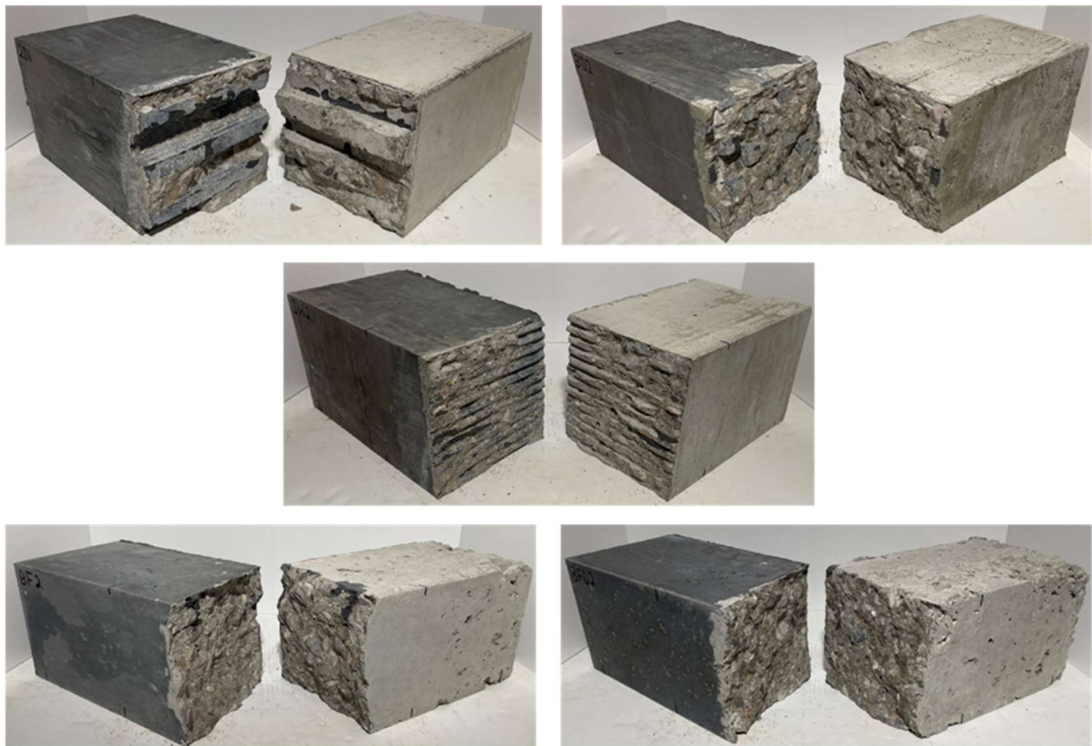
Figure 3.12: Typical MOR failures for each interface type 3
