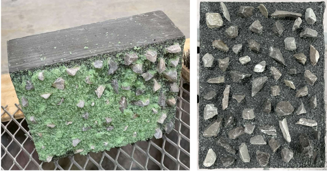
Figure A.4: Exposed Aggregate foam removal (left) and resulting texture pattern (right)
