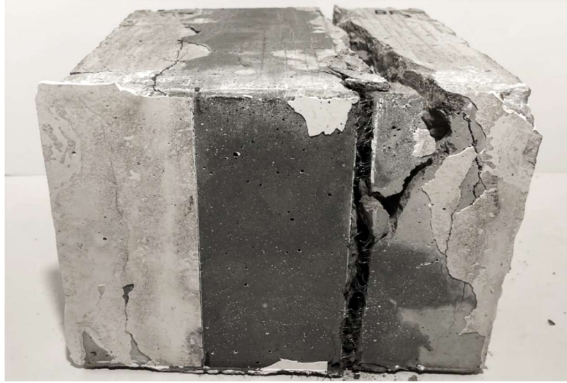
Figure 3.7: Bottom bearing surface of BiFluid specimen No. 3 2
