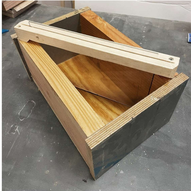
Figure 3.2: BiFluid with Divider assembly for slant shear specimen
