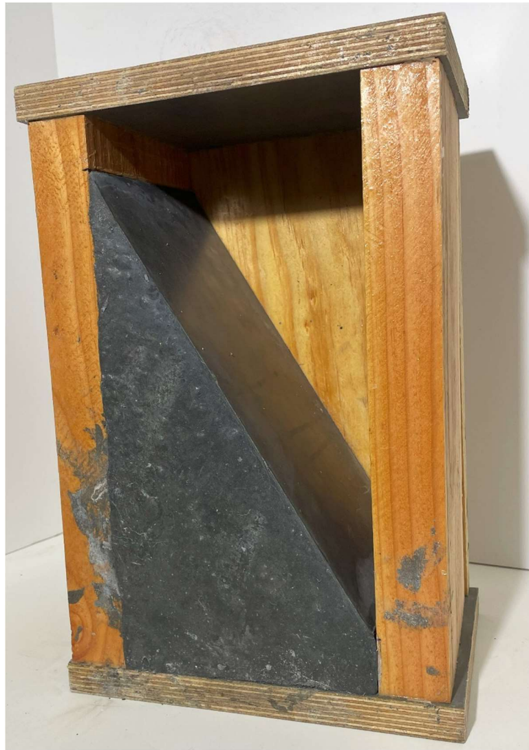
Figure A.6: Slant-Shear Specimen with a Smooth Interface texture
