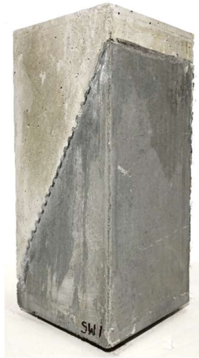
Figure 3.9: Slant shear specimen with Sine Wave interface
