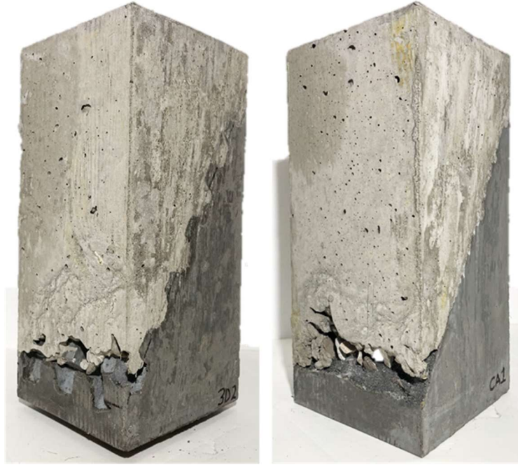
Figure 3.10: Unconsolidated areas of slant shear specimens
