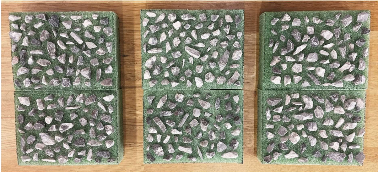
Figure 3.6: Exposed aggregate interface molds for direct shear specimens
