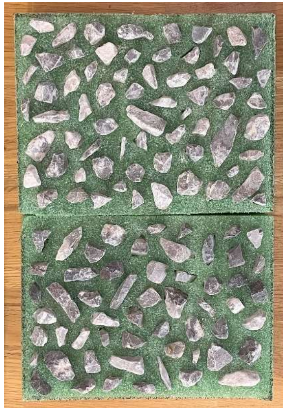
Figure A.3: Exposed Aggregates in Foam Boards
