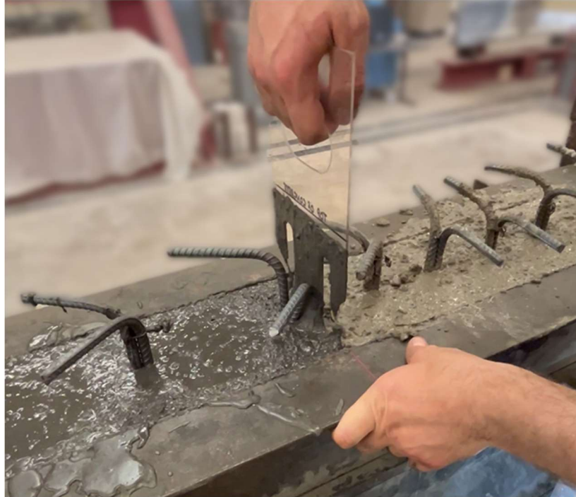
Figure 4.9: Removal of divider immediately after casting the second BiFluid with Divider girder
