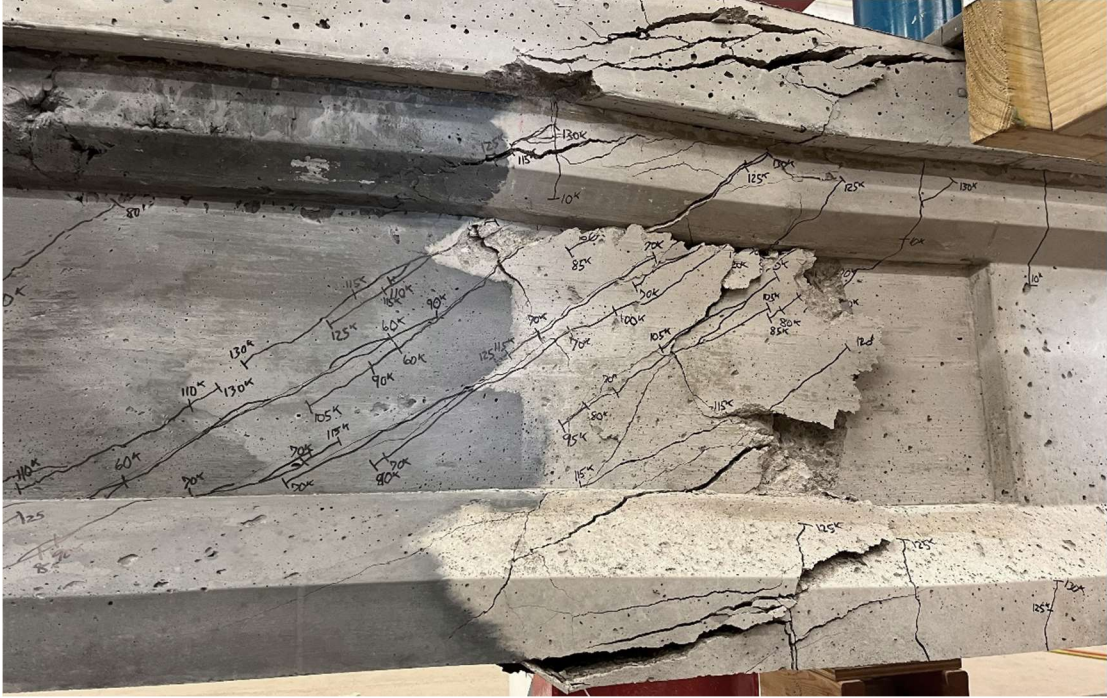
Figure 4.15: Failure of BiFluid hybrid girder no. 1
