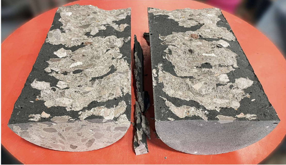
Figure 3.4: Two halves of tested BiFluid splitting-tensile specimen
