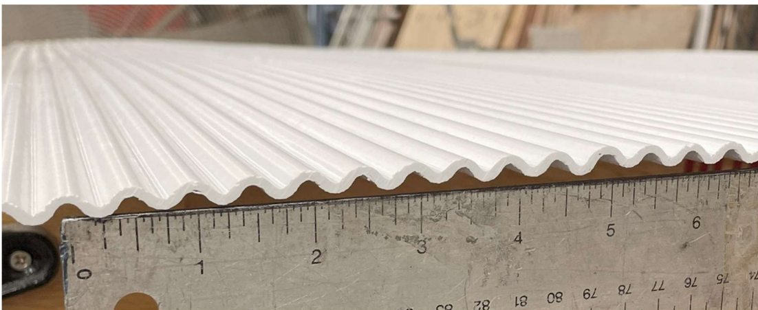
Figure A.5: Sine Wave interface form liner
