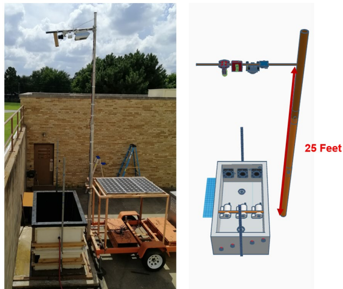
Figure 8. Water-side setup using adjustable pole.
