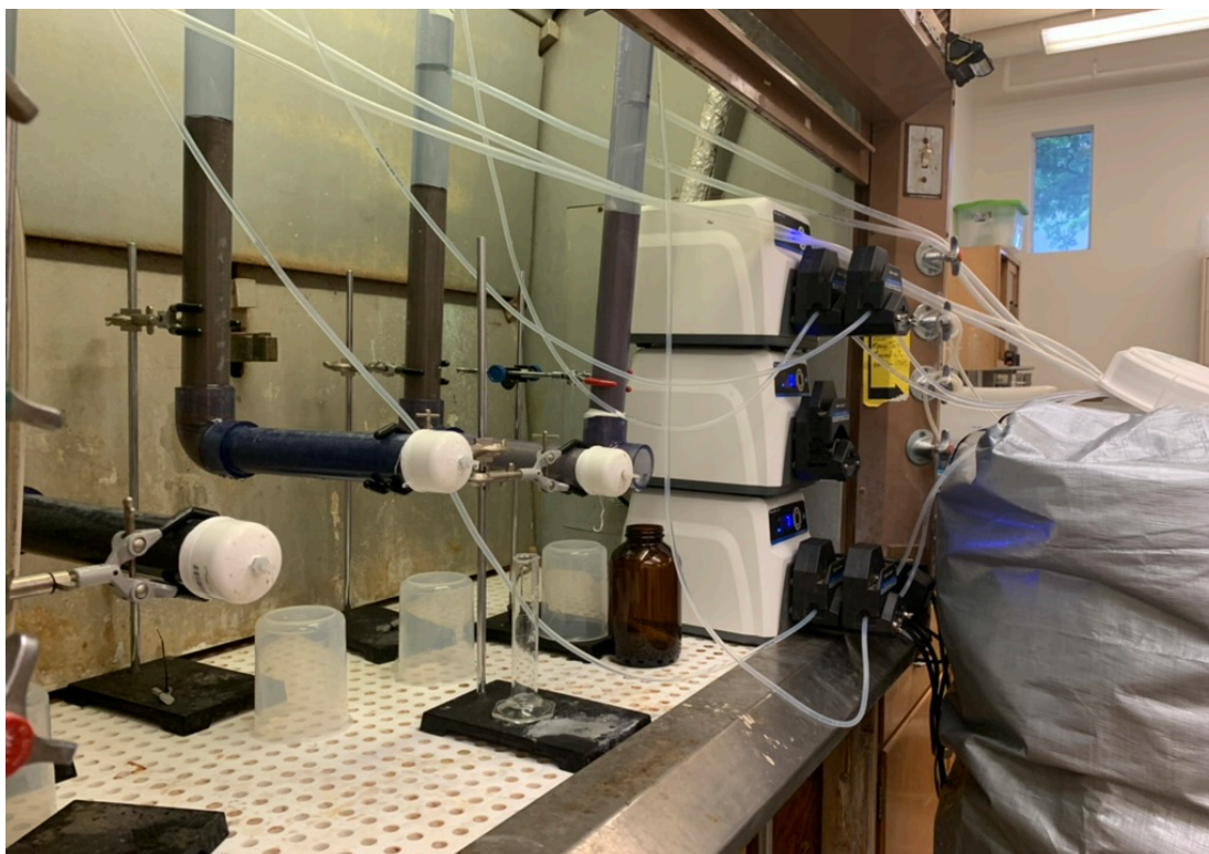
Figure 2-2 Photograph of the horizontal column setup. Pictured from left to right are the experimental columns, peristaltic pumps, and the synthetic stormwater influent tank. Experimental columns each demonstrate 6 inches of ponding in the upper portion of the vertical tube followed by 12 inches of bioretention simulation sand, a 90 degree elbow, 12 inches of a media packed tube, and lastly a cap with a 1/16 inch orifice outlet.
