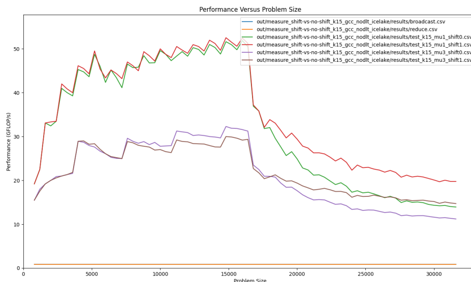
Figure 5.15: Run on an Intel Xeon Gold 6338 and compiled with GCC. This shows that there is not much difference between using the shift version of the kernel compared to noin-shift. The performance differences here are because of choosing different mu values.
