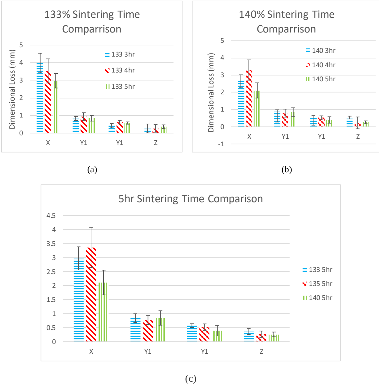
Figure 3.7 (a) 133% sintering time comparison: 3hr, 4hr, and 5hr; (b) 140% sintering time comparison: 3hr, 4hr, and 5hr; (c) 5 hour sintering time comparison between flow rates: 133%, 135%, and 140%.
