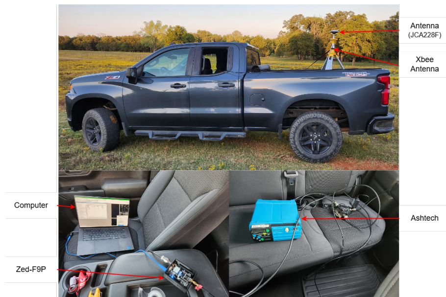
Figure 2.8. Photo of the Rover Station Setup, showing the antenna, Ashtech, ZED-F9P, Computer, and Xbee radio
