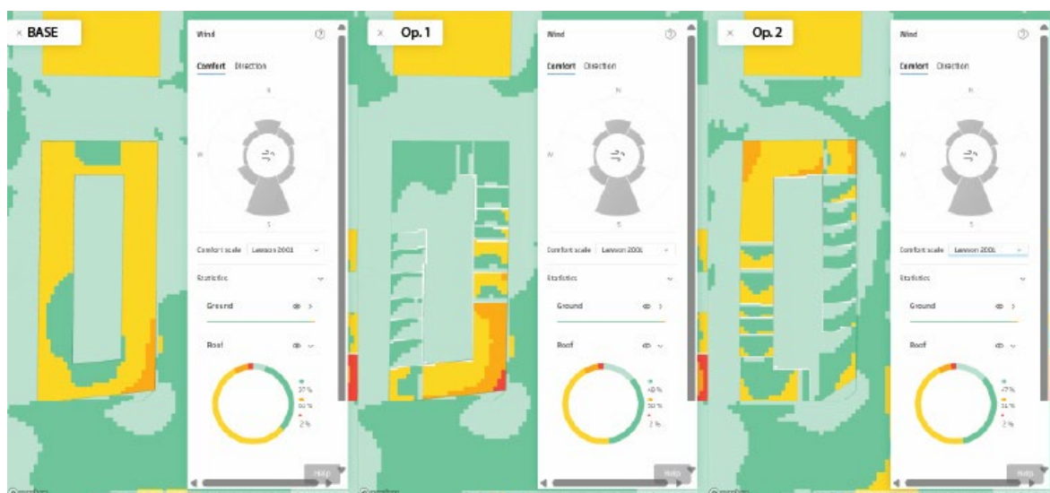
Figure 25. detailed wind performance analysis results for Option 1, 2 and base.
