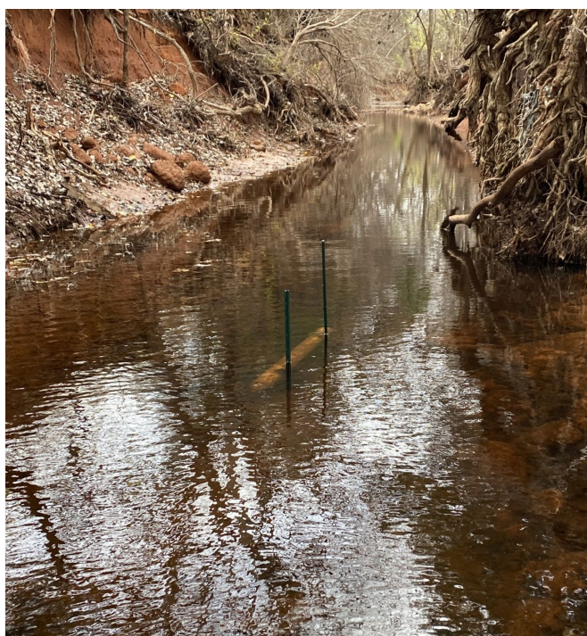
Figure 16: Passive sediment trap deployed in Dave Blue Creek
