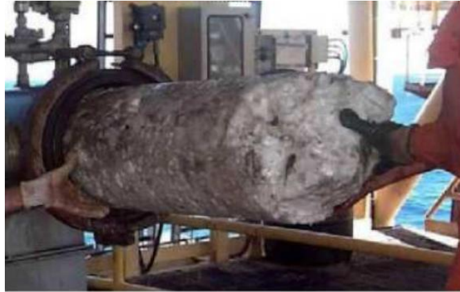
Figure 2-2. Hydrate formation in natural gas transmission pipeline (Zarinabadi & Samimi, 2012)
