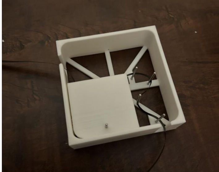
Figure 8: Printer head design with the additional pin to help introduce tension to the system.
