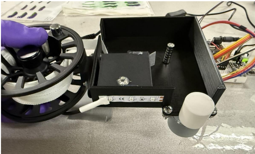
Figure 16: Underside of the printer head showing the UV light strip.
