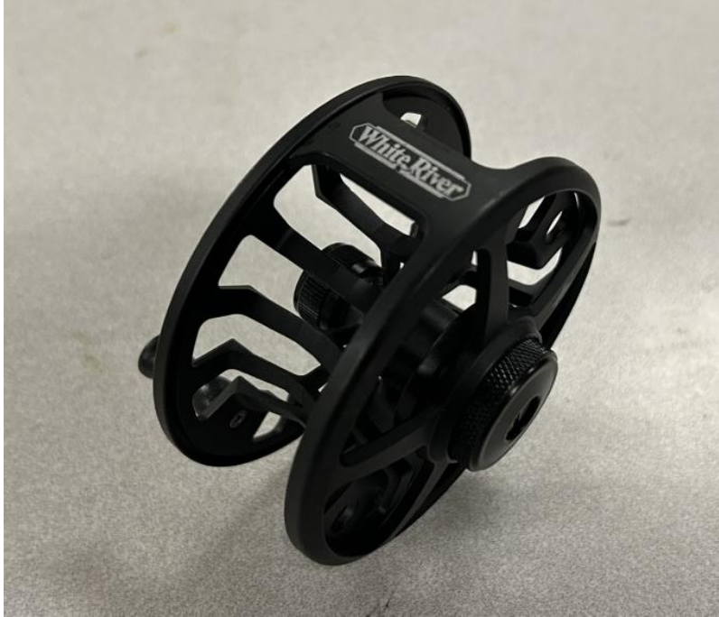
Figure 9: Fly fishing reel that will hold the fiber and create tension within the system.
