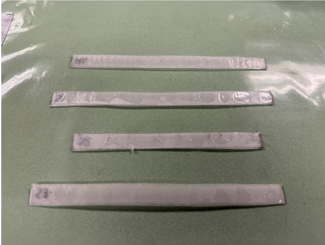
Figure 20: Back of the fiberglass composite samples to show pooling of epoxy. They are in the same order from top to bottom as Figure 19.
