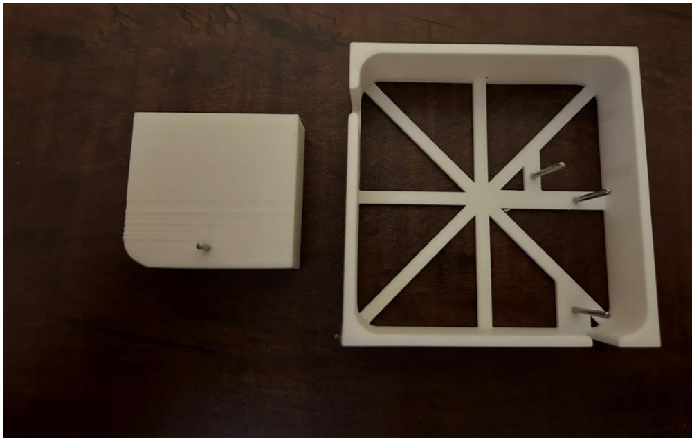
Figure 7: 3D printed truss shell with pins and epoxy reservoir.
